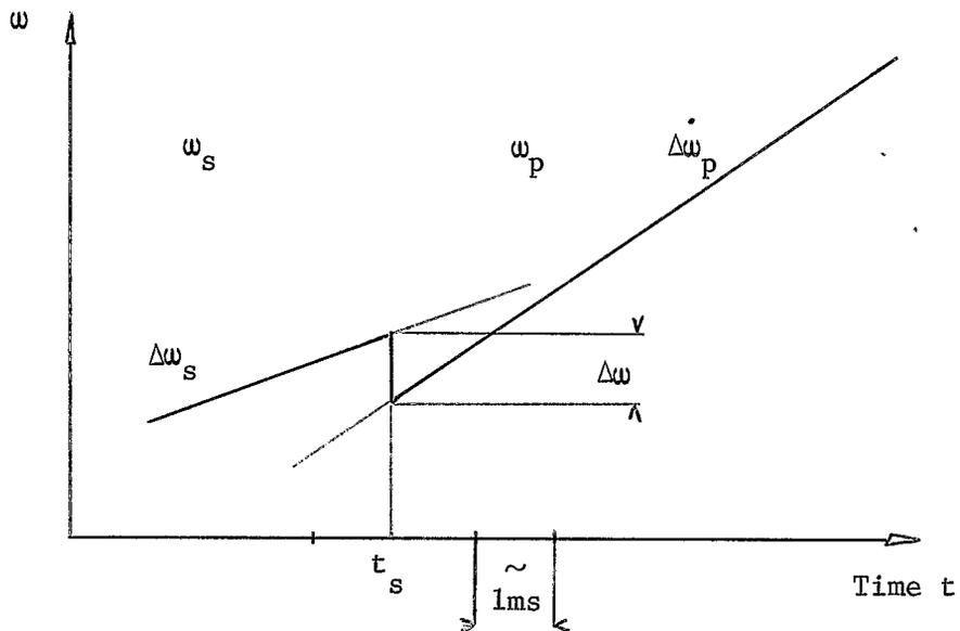
Fig. 6: Frequency Jump at the Switching Time.
