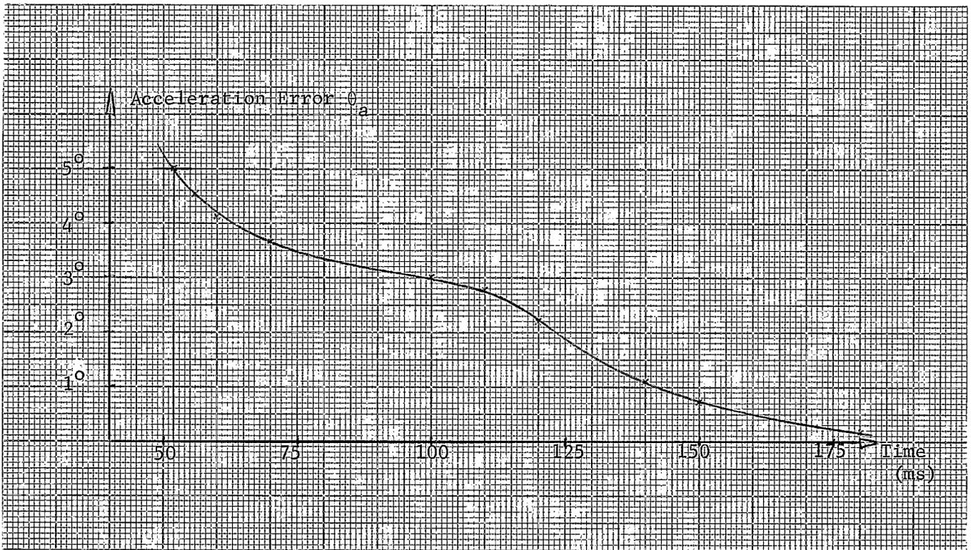
Fig. 5: Acceleration Error  $\theta_a$  vs. Time in Tracking of the RF Signal from the Pick-up Electrode.
