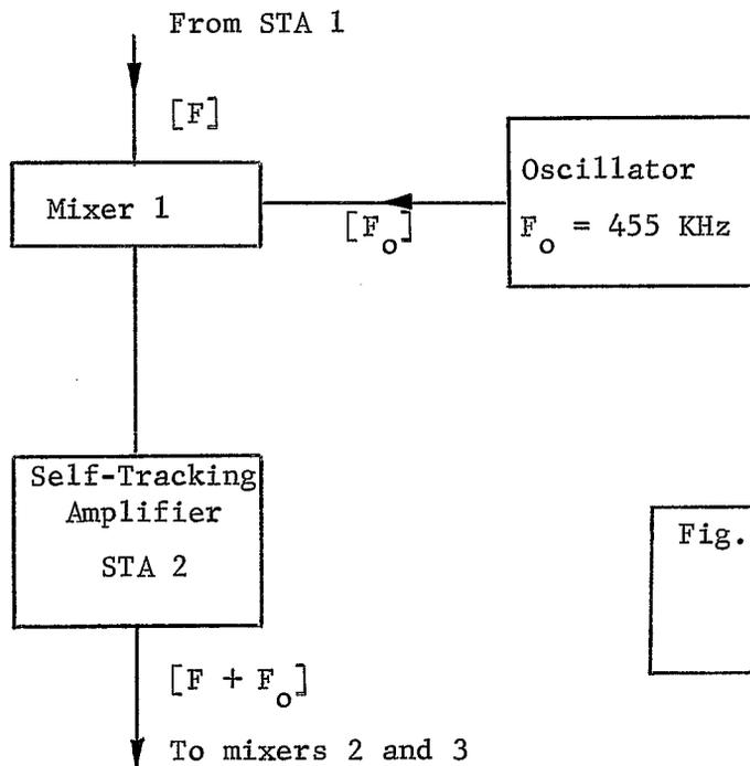
Fig. 1: Block diagram of a part of the present rf low level of the AGS.
