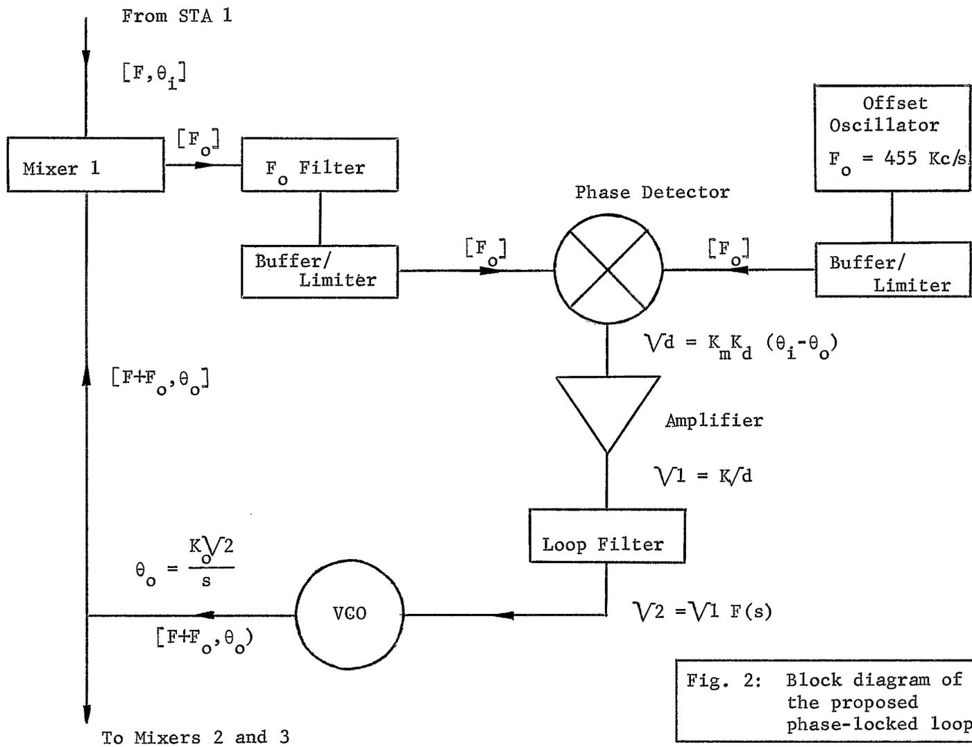
Fig. 2: Block diagram of the proposed phase-locked loop.
