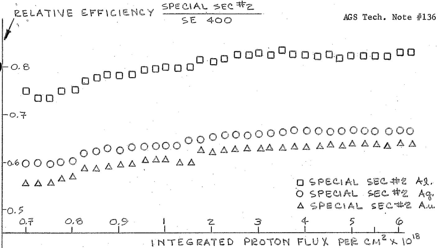
FIG. 5 RELATIVE EFFICIENCY OF SPECIAL SEC #2 AGAINST INTEGRATED PROTON FLUX PER CM<sup>2</sup> THAT TRAVERSED THE CHAMBER.
