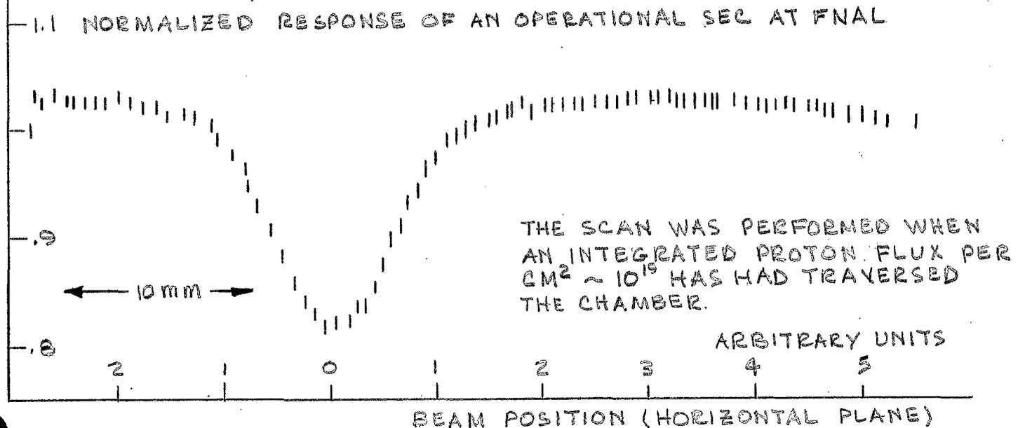
FIG. 8 NORMALIZED SEM(?) RESPONSE AGAINST RELATIVE POSITION OF THE BEAM SPOT IN THE HORIZONTAL PLANE. AS REPORTED BY F. HORNSTRA.<sup>3</sup>
