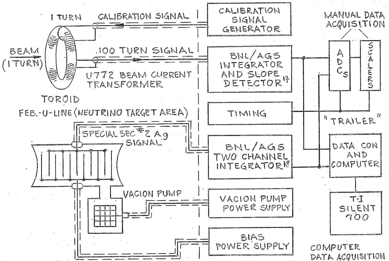
FIG. 10 HOOK UP OF THE TESTS AT BNL/AGS
