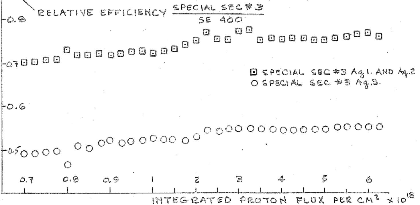
FIG. 6 RELATIVE EFFICIENCY OF SPECIAL SEC #3 AGAINST INTEGRATED PROTON FLUX PER CM<sup>2</sup> THAT TRAVERSED THE CHAMBER.
