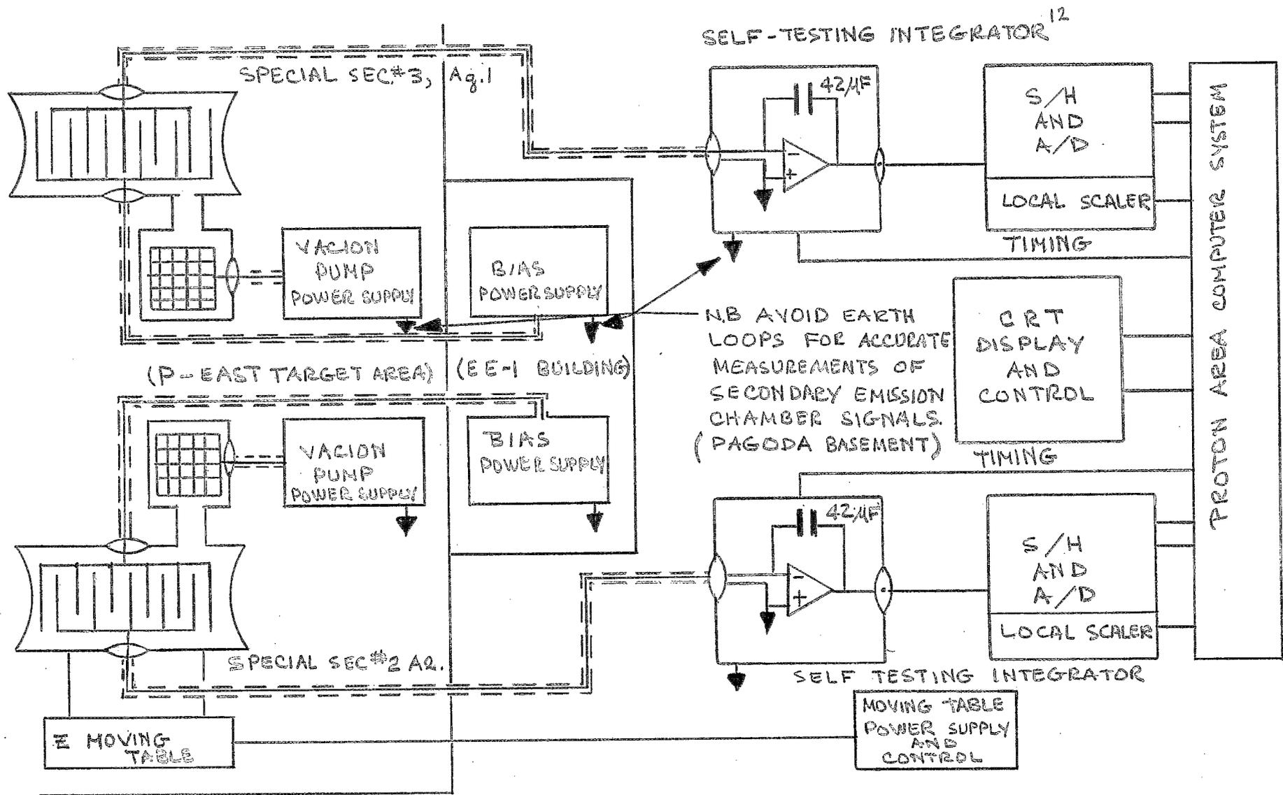
FIG 4. HOOK UP OF THE SPECIAL SECONDARY EMISSION CHAMBERS AT FNAL.
