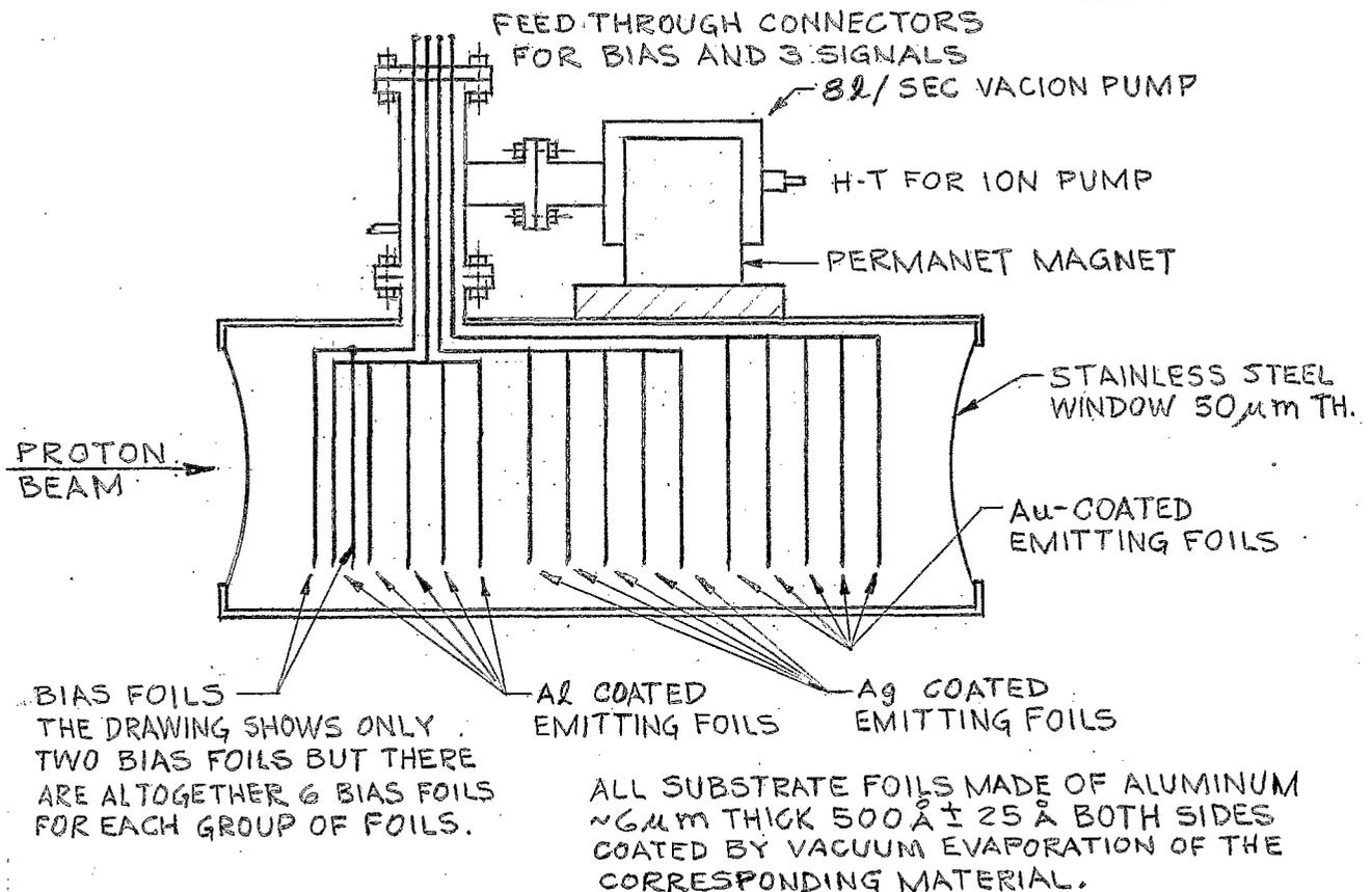
FIG. 1 A SIMPLIFIED DRAWING OF THE SPECIAL SEC #2
