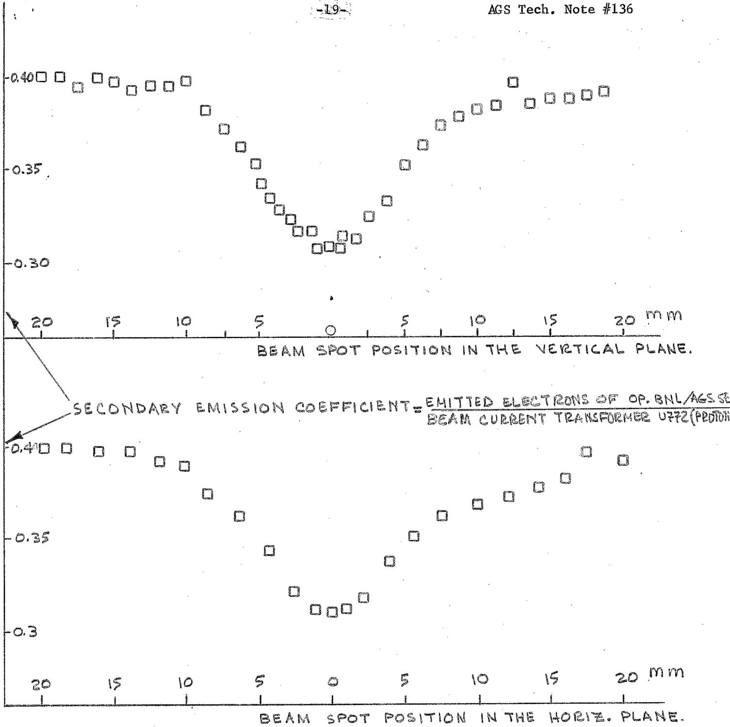
FIG. 13. SECONDARY EMISSION COEFFICIENT OF THE BNL/AGS OPERATIONAL SEC AGAINST BEAM SPOT POSITION IN FEB.
