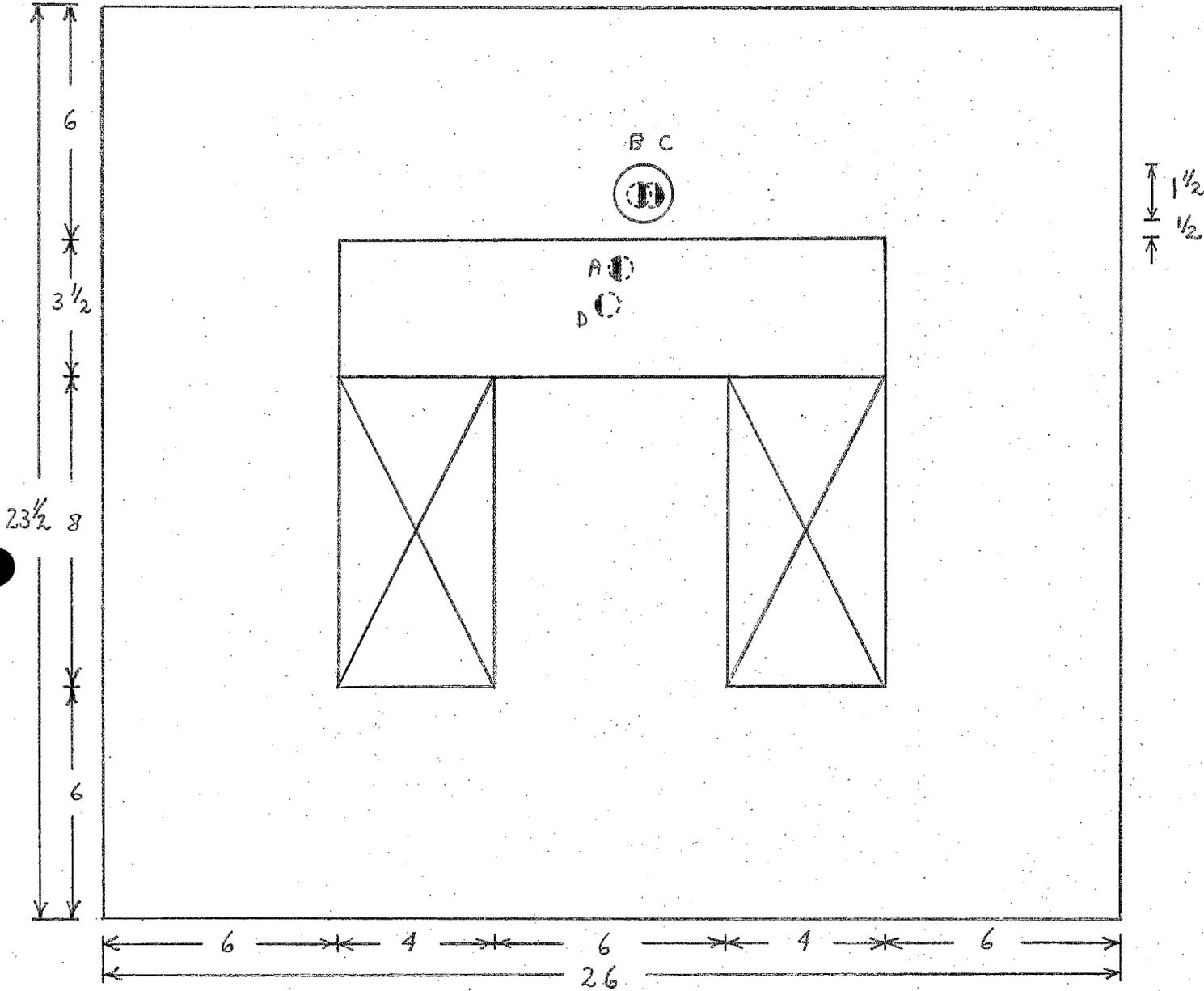
Fig. 4 - Upstream view of Lambertson magnet L<sub>3</sub>, showing the four beam components that enter it. This magnet bends the D and A beams to the left.
