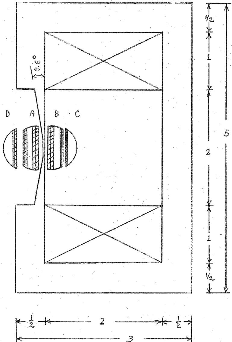
Fig. 3 - Upstream view of Lambertson magnet  $L_1$ , showing the four horizontally split beam components. The striped areas of the beam components indicate the effect of beam divergence on the septum shadows. This magnet bends the B and C beams up.
