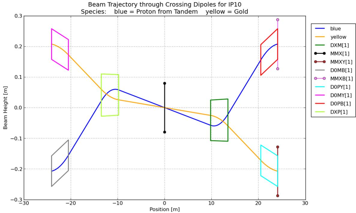
Figure 2. A non-colliding insertion. The crossing angle is  $-0.3305\text{mrad}$ . The beam trajectory is  $59.8\text{mm}$  from the central axes for both beams in the DX magnet. The Blue beam reaches its peak at  $10.5\text{m}$  from the IP, while the Yellow beam reaches its peak at  $13.5\text{m}$  from the IP.
