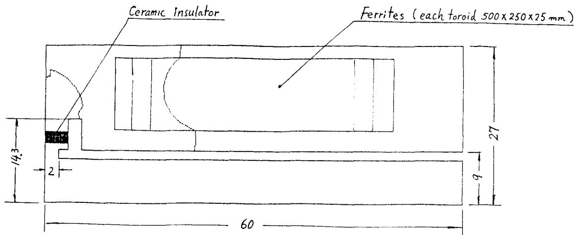
Fig.2 Main dimension of a quarter of cavity
