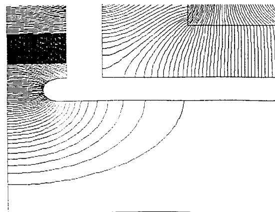
Fig.4 Electric field distribution with different shapes of accelerating electrode
