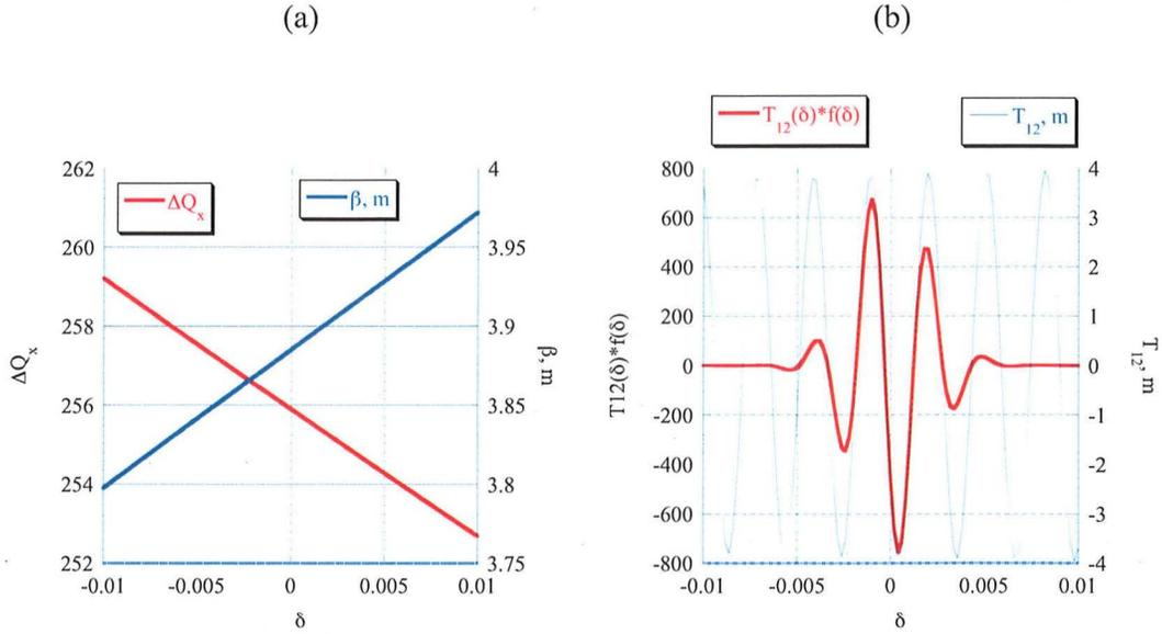
Figure 9. The FODO beam-line optics parameters as function of the particle momentum for a nominal tune advance per cell  $\Delta Q_x(\delta = 0) = 0.2499$ : (a) Dependence of the total horizontal tune advance (red line) and beta-function (blue line) on the relative momentum deviation  $\delta$ ; (b) Dependence of the beam-line's  $T_{12}$  element (blue line) and its convolution with the momentum distribution function (red line) on the relative momentum deviation  $\delta$ .
