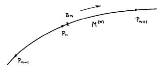
The above drawing displays the particle trajectory through the three points of interest. Consider what is happening at the n-th beam position monitor and its two immediate neighbors. We label the monitor/ corrector block by  $P_m$  and the phase space point at  $P_m$  by  $X_m$ , i.e.  $X_m$  will be the following column vector
