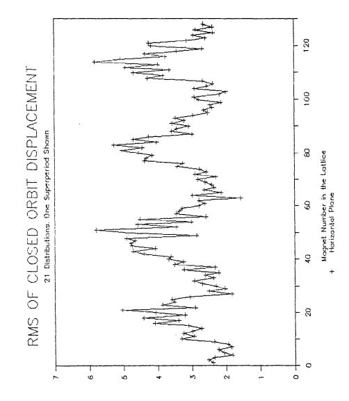
RMS Of CO Displacement (mm)
