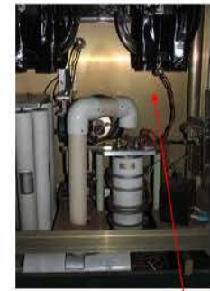
Front view, with cover removed, of blue kicker #1. General area dose rates: 0.8 to 1.7mR/Hr
