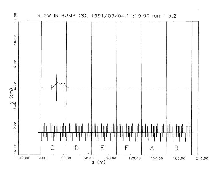
Fig.2. FIB = Fast Injection Bump. Horizontal, order-3. x = -25 mm, resulting x' = 3.474 mrad.
