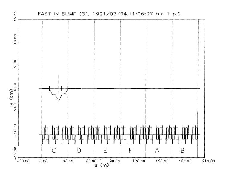
Fig.3. HIB4 = Fine Injection Bump. Horizontal, order-4. x = 1 mm, x' = 0.
