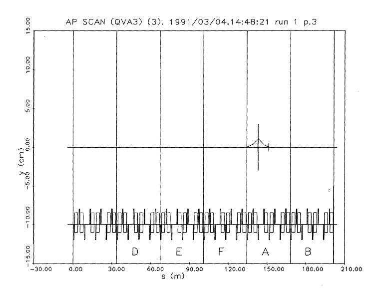
Fig. 5. ASQHA4 = Aperture Scan on Even Quadrupole. Horizontal, order-3. y = 10 mm, resulting y' = -1.671 mrad.
