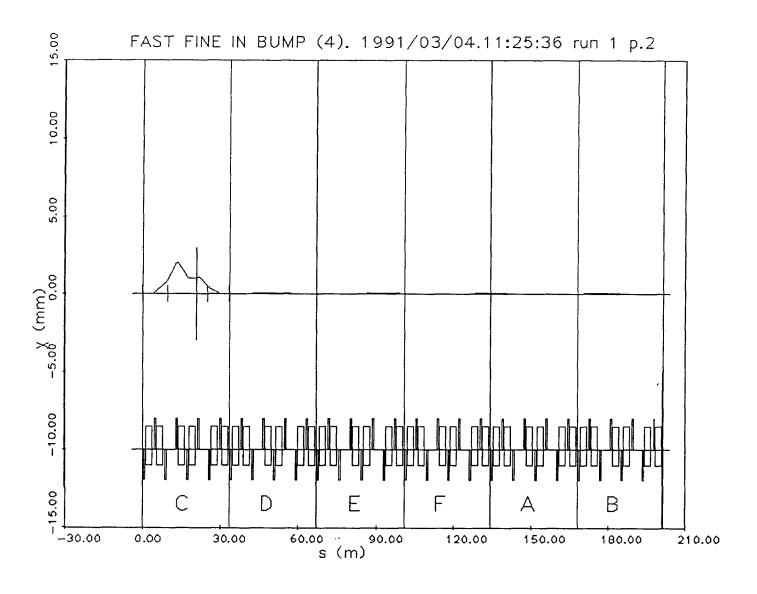
Fig.4. ASQVA3 = Aperture Scan on Odd Quadrupole. Vertical, order-3. y = 10 mm, resulting y' = -1.744 mrad.
