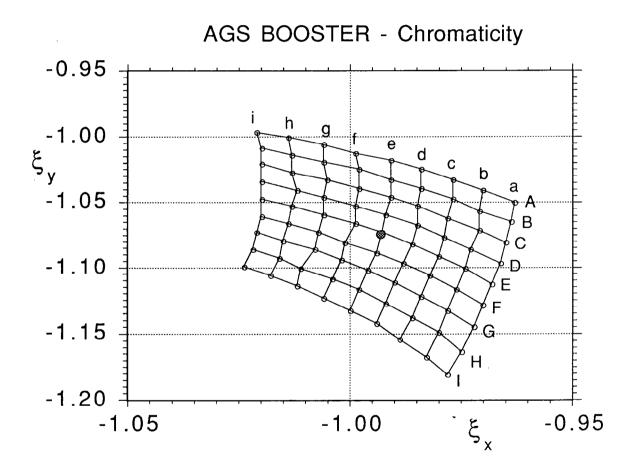
Fig. 7. Chromaticity for protons at extraction, by varying quadrupoles (table V).
