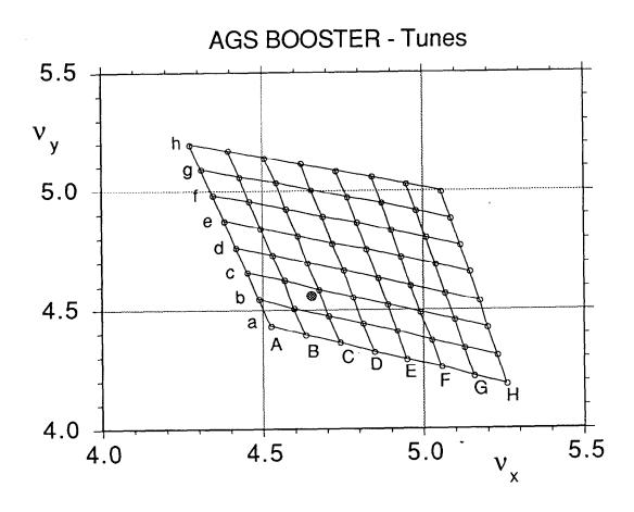
Fig. 3. Tune chart for protons at injection, by varying quadrupoles (table III).
