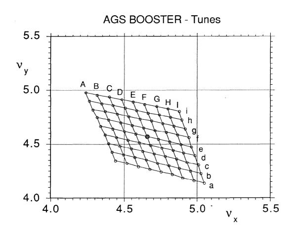
Fig. 6. Tune for protons at extraction, by varying quadrupoles (table V). The bare machine value at injection is marked by the gray dot.
