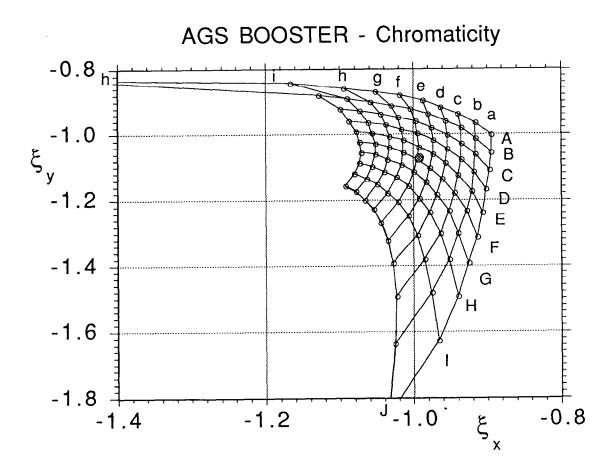
Fig. 2. Chromaticity for protons at injection, by varying quadrupoles (table II). The bare machine value at injection is marked by the gray dot.
