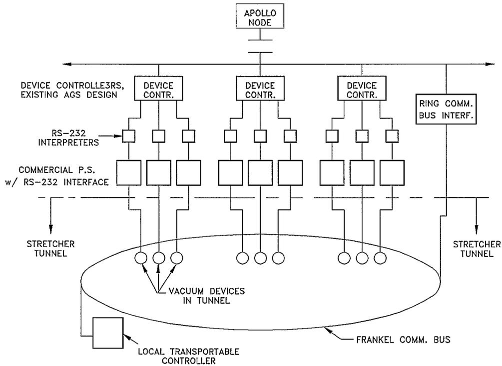
Figure 7. Stretcher Vacuum Instrumentation and Control System
