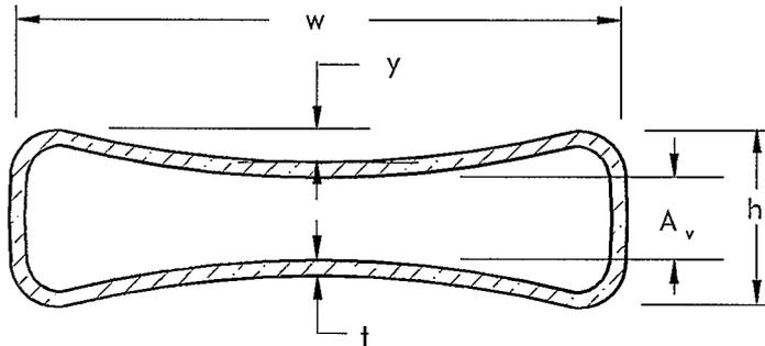
Figure 3. Strain In Dipole Chamber Due To Atmospheric Pressure
