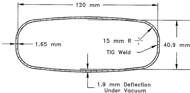
Figure 4. Required Dipole Chamber Shape For Maximum Vertical Beam Aperture When Chamber Is Strained By Vacuum Loading
