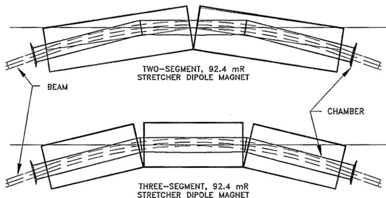
Figure 1. Three-Segment Beam Chamber
