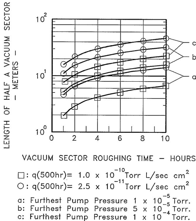
Figure 5. Pressure at the Sputter-Ion Pump Furthest Removed From the Sector Roughing Pump as a Function of Time and Assumed Beam Pipe Outgassing Rates.
