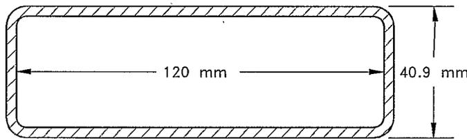
The effects of external pressure on the chamber deflection is represented by strain in the chamber shown in Fig. 3. This assumes that the chamber is not pre-stressed. The maximum vertical aperture,  $A_v$ , is:
