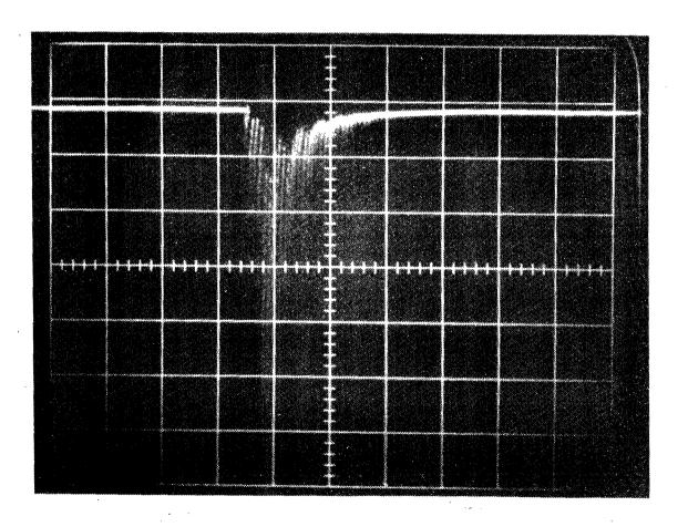
Fig. 1 Fast-slow spill induced by 20 nsec, 43 kV fast kicker pulse. Detector was lucite Cerenkov counter with 470 determination viewing R20 collimator in slow external beam. Oscilloscope horizontal sweep rate is 100 psec/div.
