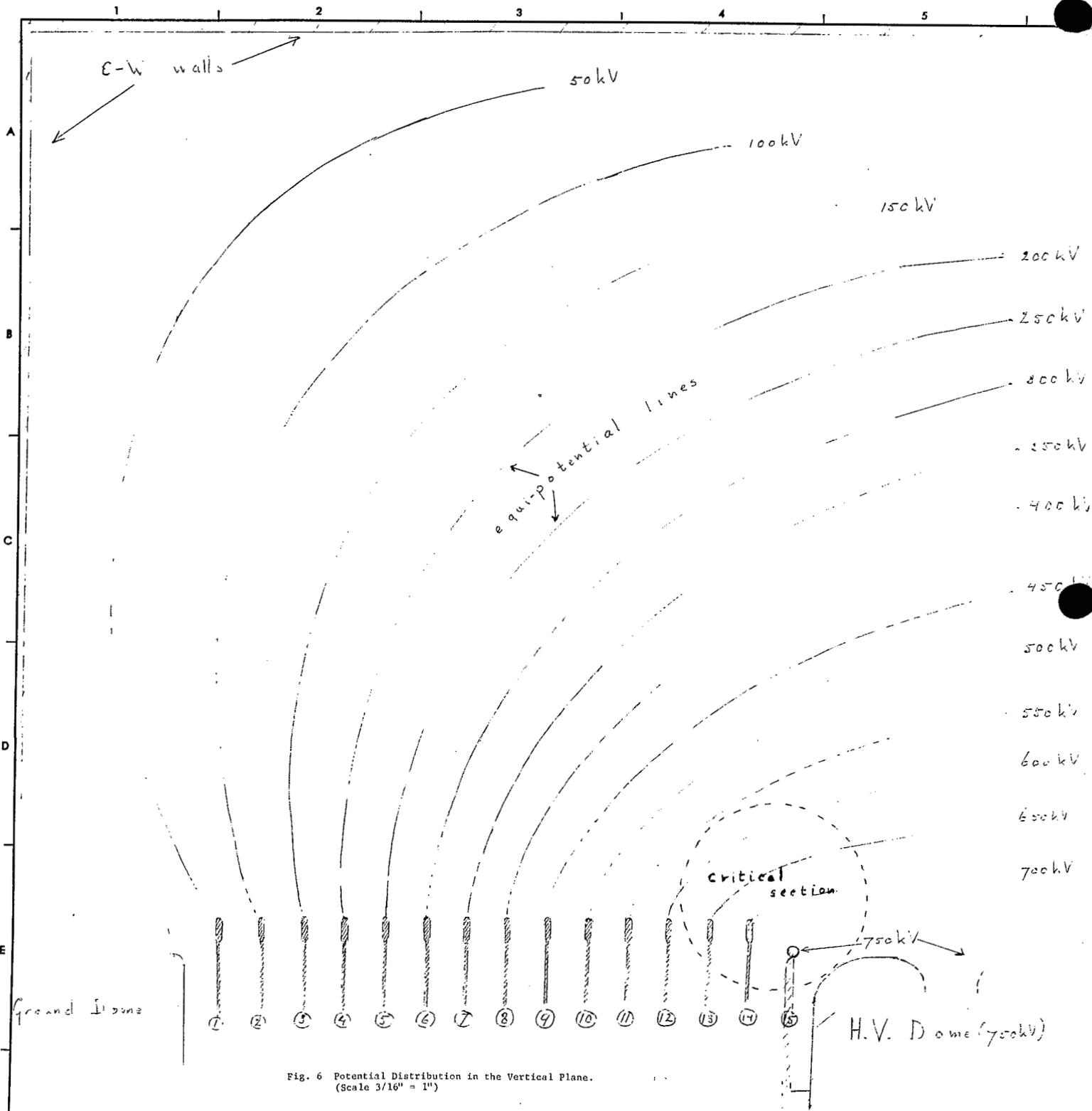
Fig. 6 Potential Distribution in the Vertical Plane.
