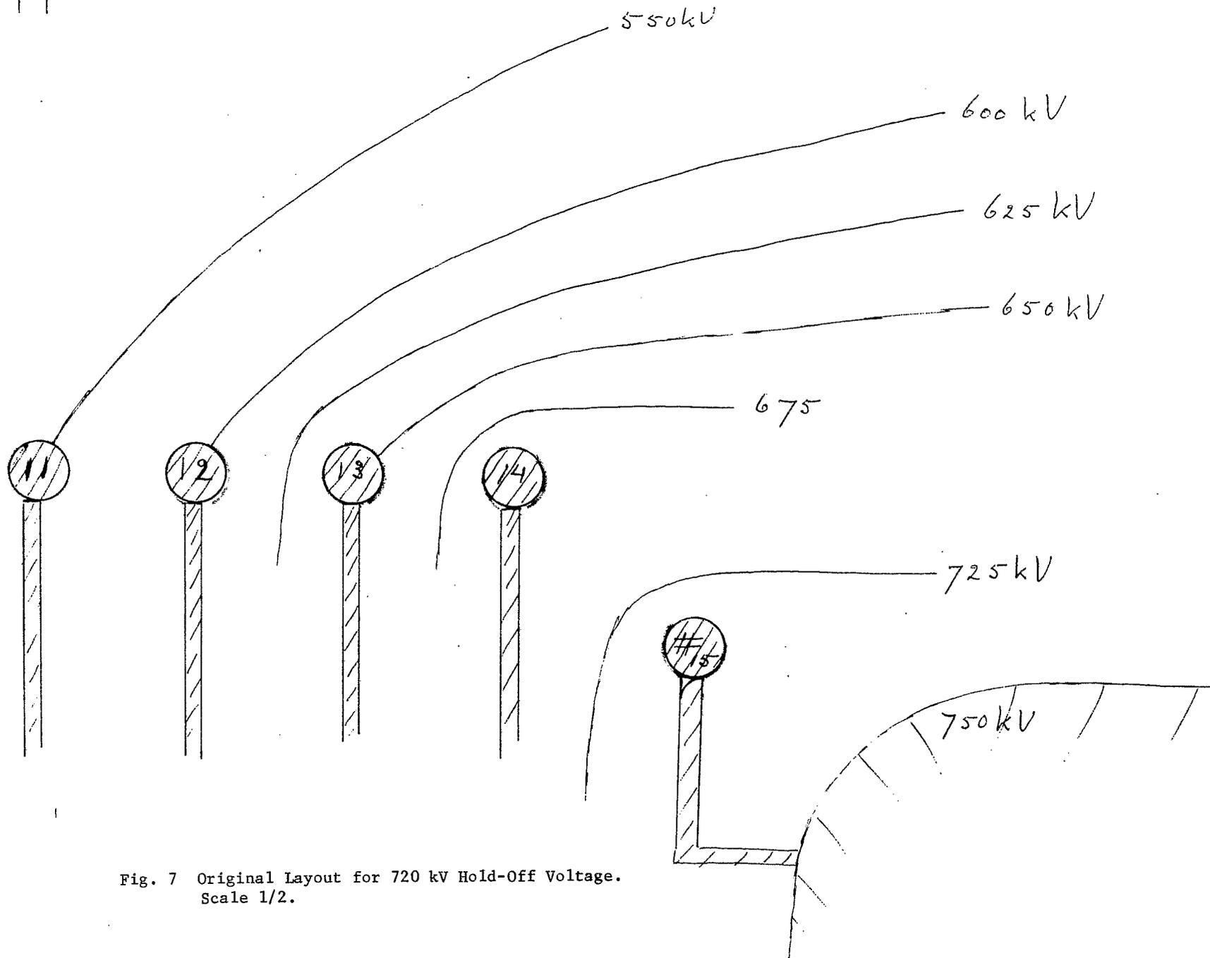
Fig. 7 Original Layout for 720 kV Hold-Off Voltage.
