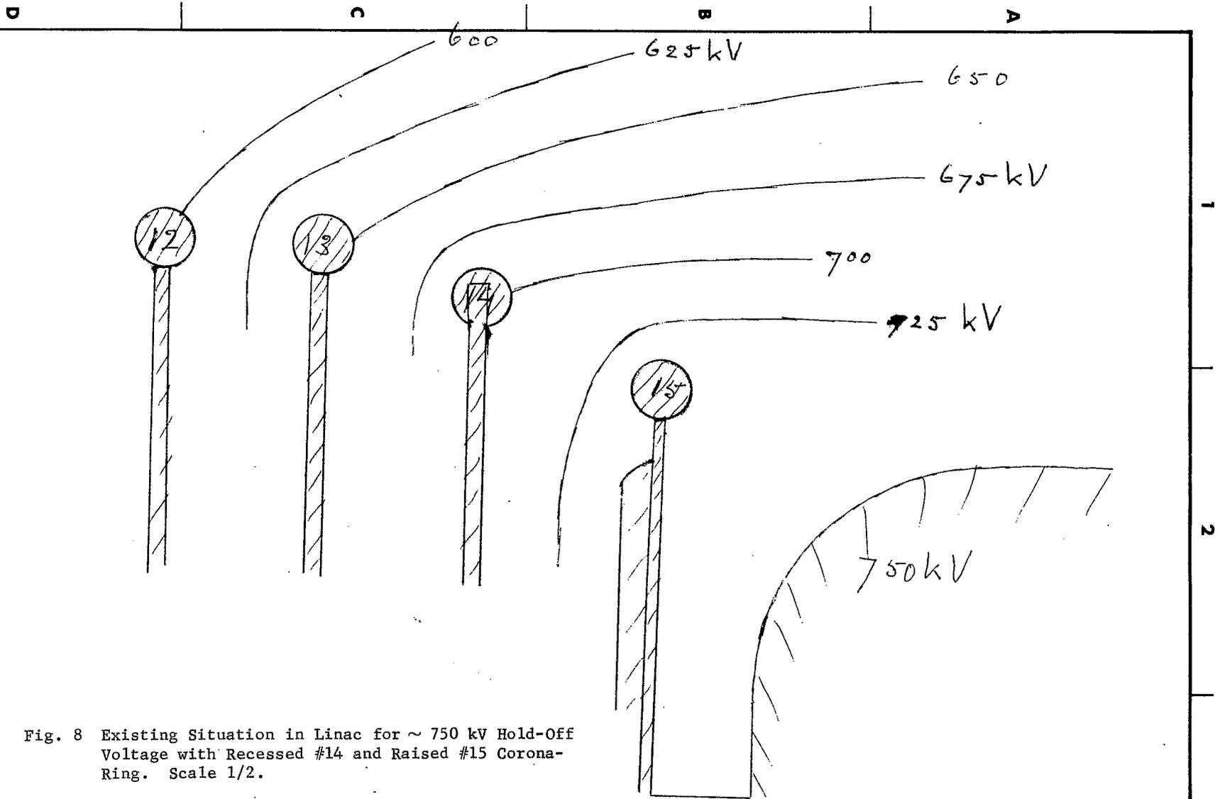
Fig. 8 Existing Situation in Linac for ~ 750 kV Hold-Off Voltage with Recessed #14 and Raised #15 Corona-Ring. Scale 1/2.
