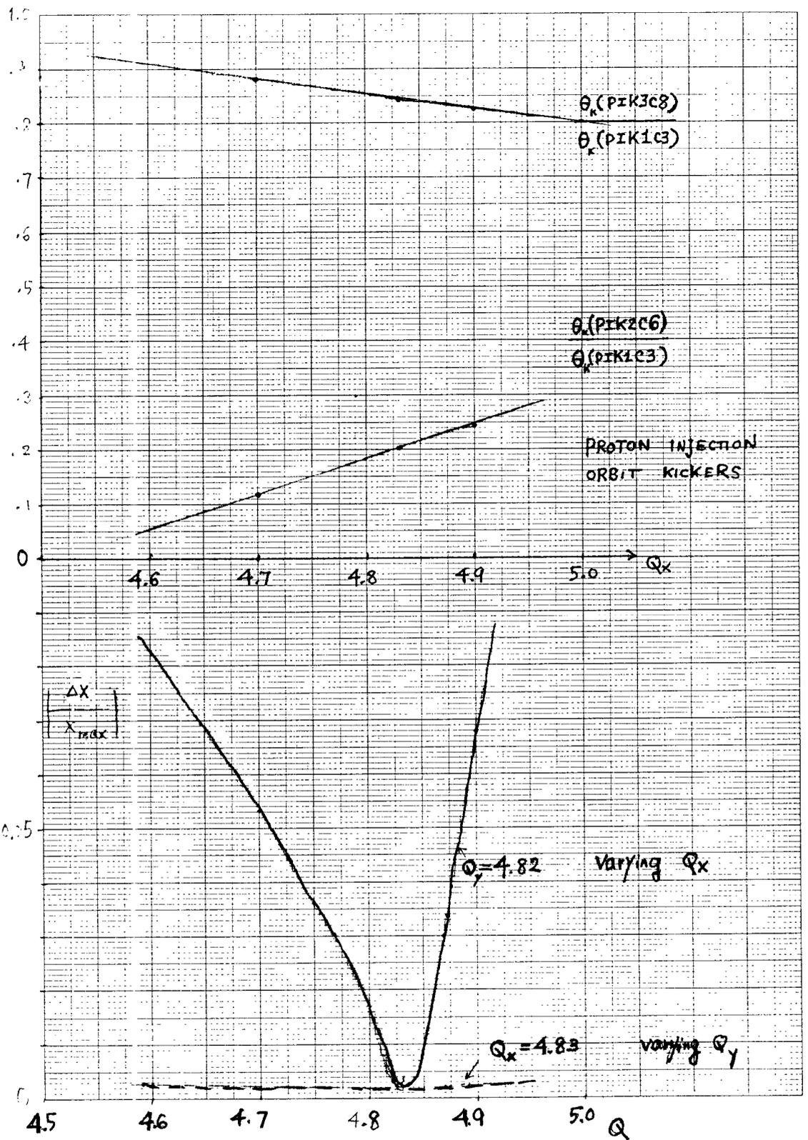
Fig. 5 Lower : Ratio of closed orbit displacement outside the bump region to the maximum displacement in the bump region is plotted as a function of tune for varying  $Q_x$  (solid) and varying  $Q_y$  (dashed line)
