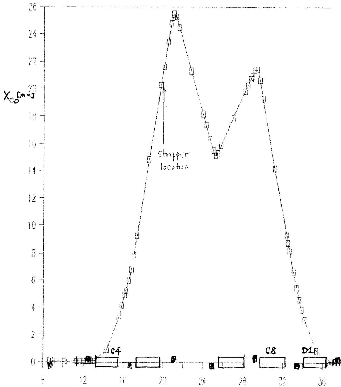
Fig. 3 Slow bump orbit for proton injection
