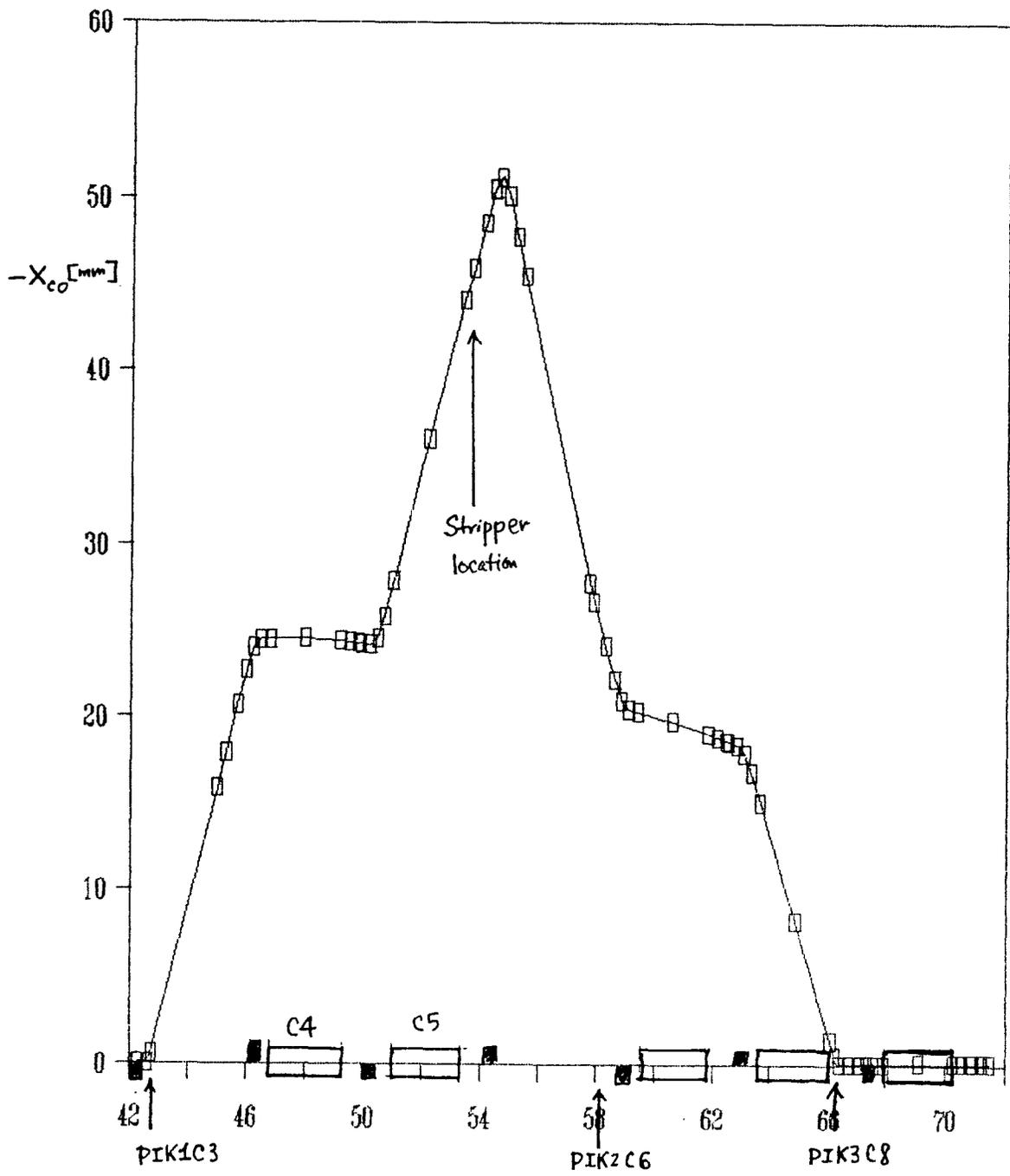
Fig. 2. Proton injection orbit bump of fast kickers
