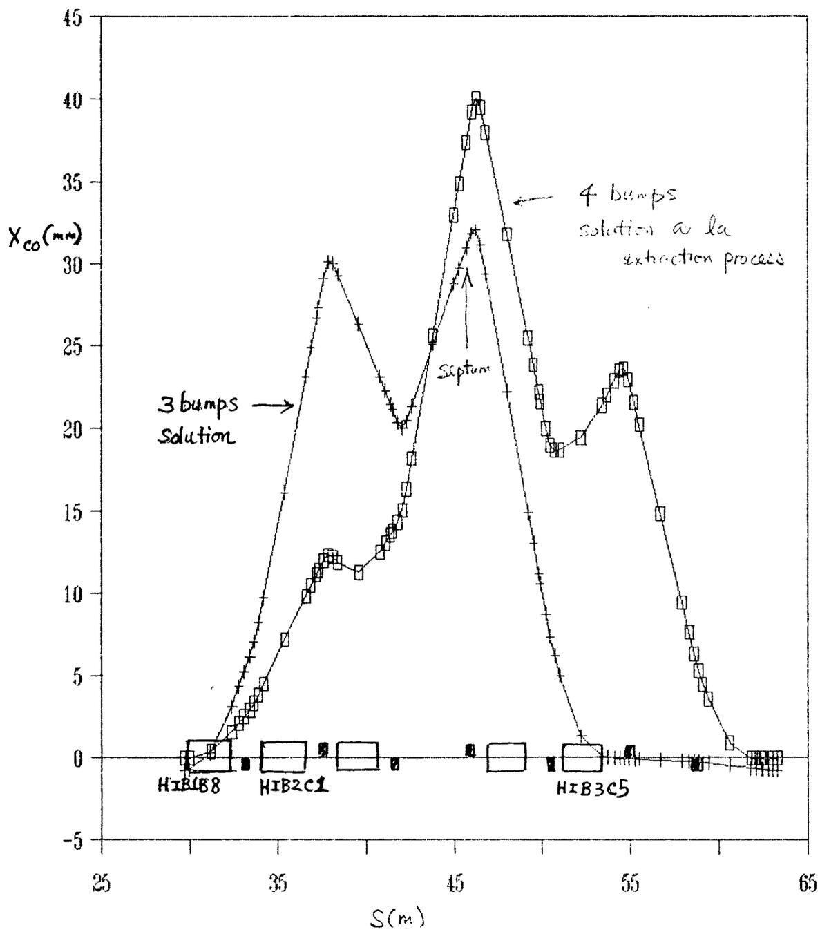
Fig.3 closed orbit of HI injection slow bumps
