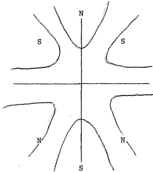
Equivalent Sextupole Produced by the 8 Degree Dipoles
