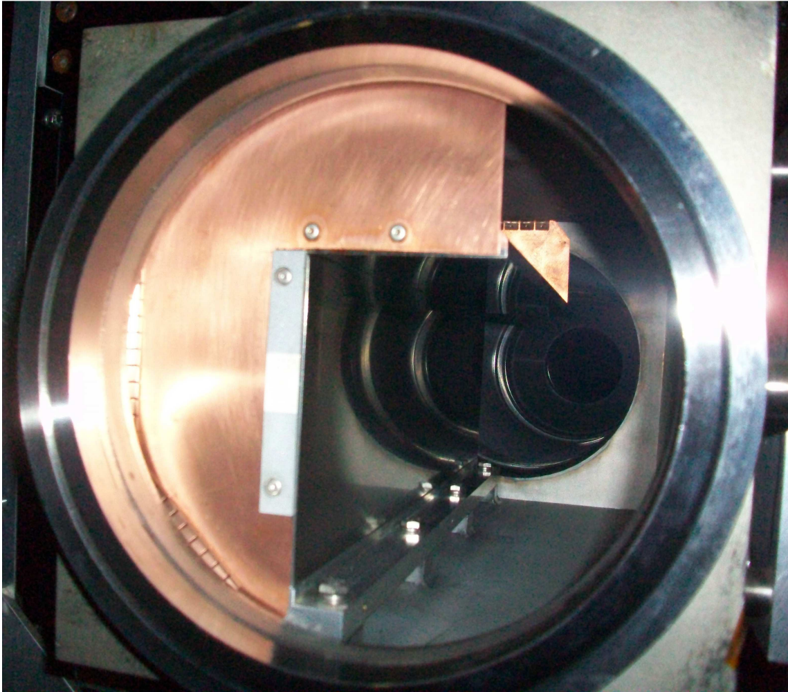
Figure 4: Recently inspected Yellow primary collimator, showing a flat surface without any damage.
