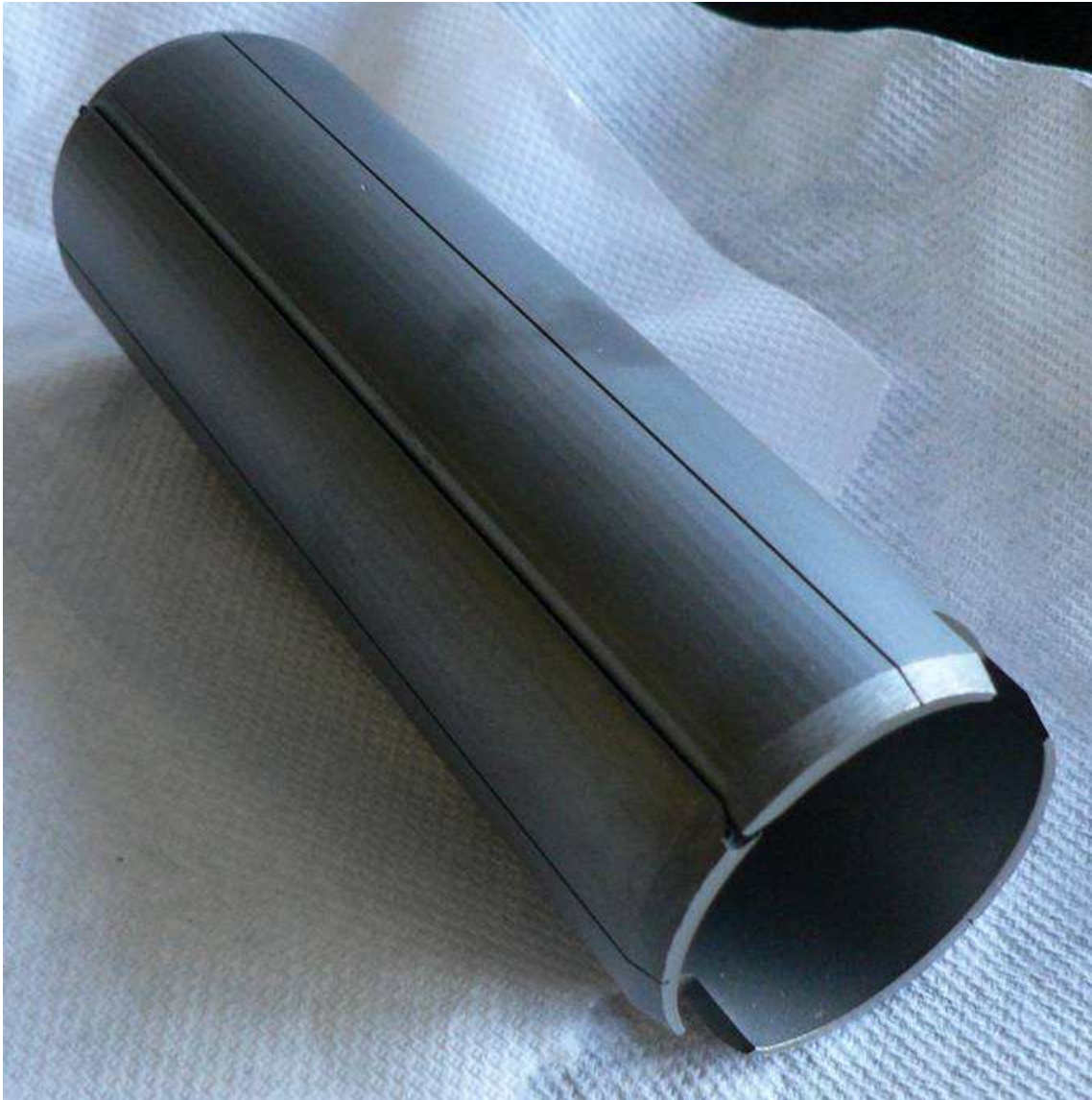
Figure 3: One of the sleeves inserted in the RHIC beam pipe adjacent to the dump to increase its wall thickness.
