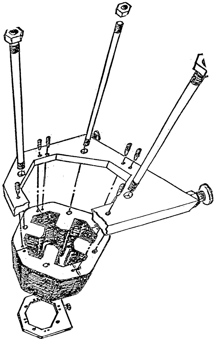
Figure 16. Quadrupole assembly.
