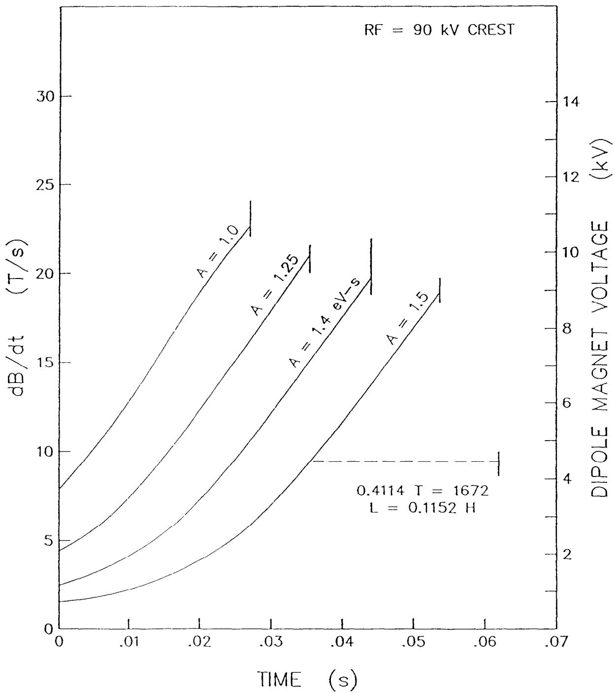
Figure 40,  $dB/dt$  and dipole voltage versus time.
