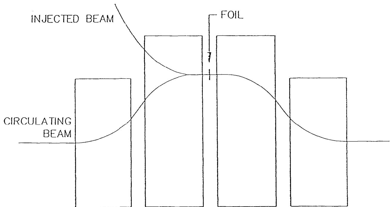
Figure 20. Bump in the circulating beam at injection.
