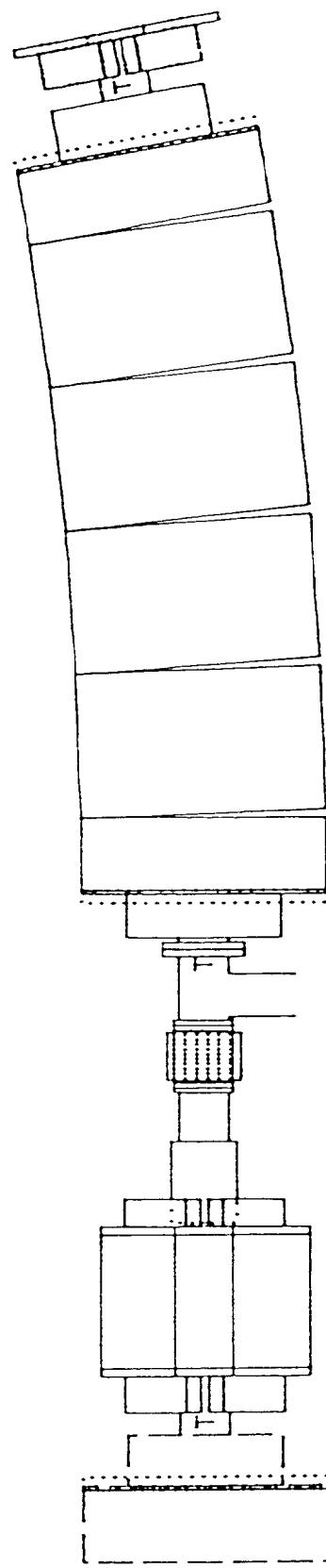
Figure 35. Half-cell 8 differs from half-cells 1, 4, and 7 only in its not having a sextupole. The CT assembly is omitted in this half-cell in super-periods C and F.
