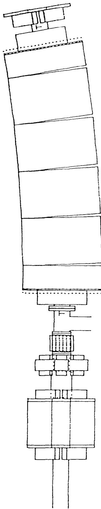
Figure 29. Half-cell 2 is followed by a straight section, thus no transition piece is required for the beam pipe downstream of the quadrupole.
