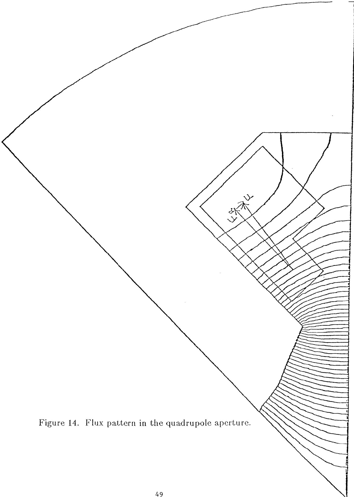
Figure 14. Flux pattern in the quadrupole aperture.
