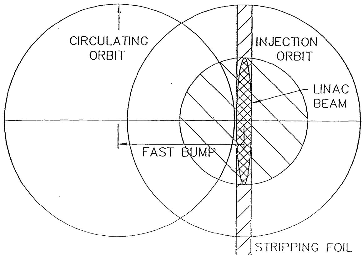
Figure 25. Injected and circulating polarized proton beams.
