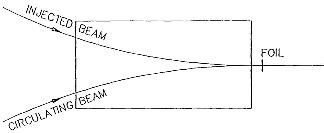
Figure 19. Foil location downstream of dipole.
