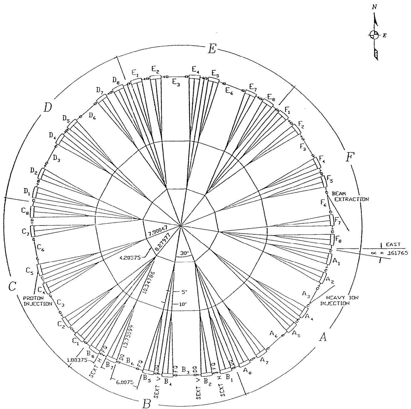
Figure 1. The layout of the Booster.
