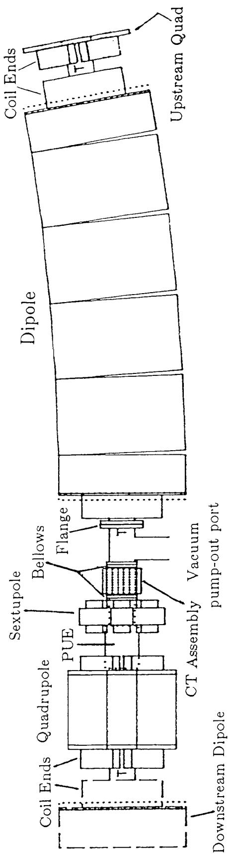
Figure 28. The first half-cell of each superperiod has, in general, a sextupole and a CT assembly in addition to the dipole and quadrupole. This half-cell is identical to half-cells 4 and 7 and differs from half-cell 2 only in its being followed by another dipole instead of being followed by a straight section.
