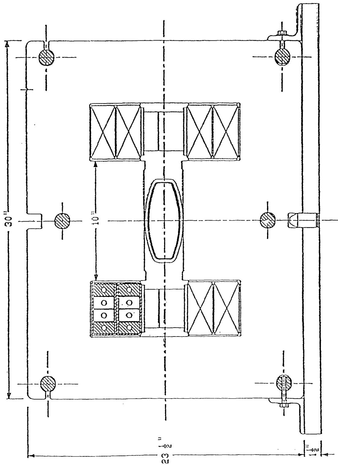
Figure 4. Dipole magnet, cross-section.
