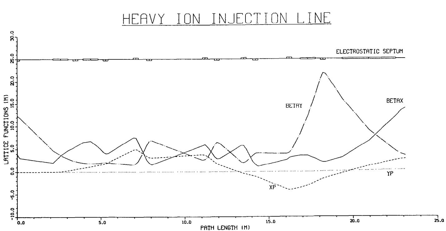
Fig 9. The optics of the heavy ion injection line.
