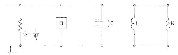
This new circuit has a parallel shunt resistance  $R_T = \frac{R\rho}{R+\rho}$  a resonant frequency  $\omega_r$  and a quality factor  $Q_L$ .
