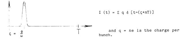
$$\begin{cases} a_n = \frac{2}{T} \int_0^T q \,\delta \,(t-\zeta) \,\cos \,2\pi n \,\frac{t}{T} \,dt = \frac{2q}{T} \,\cos \,\pi \,\frac{\zeta}{T} \\ b_n = \frac{2}{T} \int_0^T q \,\delta \,(t-\zeta) \,\sin \,2\pi n \,\frac{t}{T} \,dt = \frac{2q}{T} \,\sin \,2\pi \,\frac{\zeta}{T} \end{cases}$$
