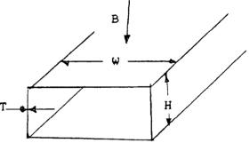
for example, if we assume B; 6.5 Tesla/sec W; .15 m (6 inches) T; 2 mm H; 3.8 cm (1.5 inches) Pside = 50 watts/m PT and B = 1.5 watts/m Ptotal = 51.5 watts/m
