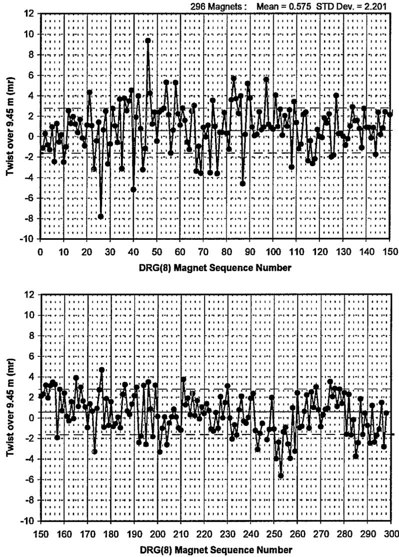
Figure 2: Average twist angle over the length of RHIC dipole magnets versus dipole magnet number. Larger twists were observed in some of the earlier magnets, which was kept better under control for the remainder of the production.
