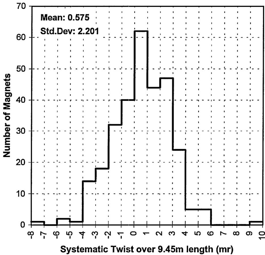
Figure 3: Distribution of average twist angles for 296 RHIC dipole magnets. The mean of the distribution is 0.58 mrad, with a standard deviation of 2.2 mrad.
