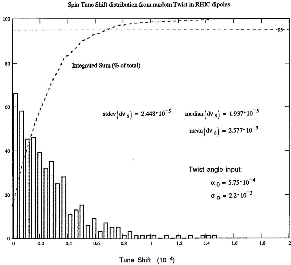
Figure 4: Distribution of spin tune shift (from the ideal value of 0.5) for an ensemble of 500 "RHIC rings." The dotted curve is the normalized integrated sum.
