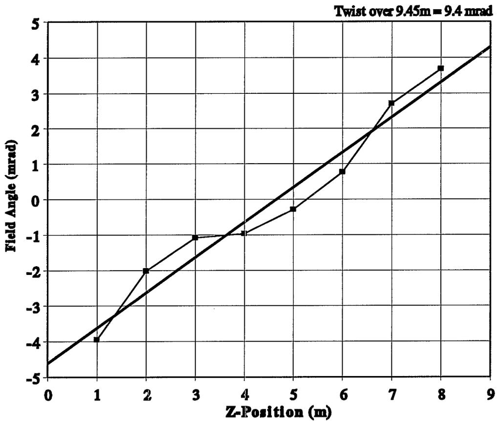
Figure 1: Field direction, in mrad from vertical, versus axial location along the length of RHIC dipole DRG516. The average twist of the field is 9.4 mrad.
