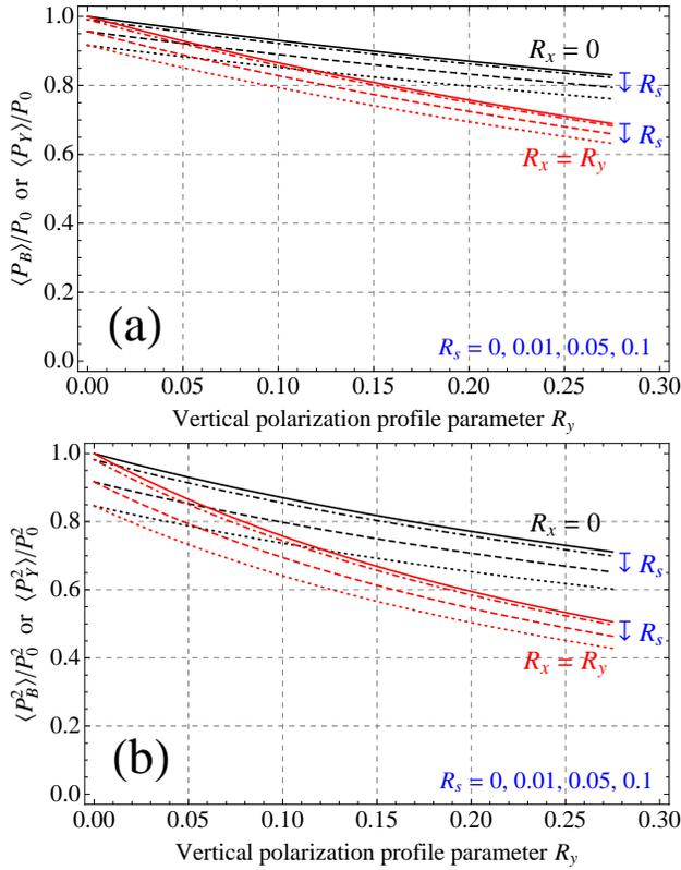
Figure 2: For single spin colliding beam experiments (a) relative reduction of the average polarization  $\langle P_B \rangle / P_0$  or  $\langle P_Y \rangle / P_0$ , and (b) relative reduction of the figure of merit  $\langle P_B^2 \rangle / P_0^2$  or  $\langle P_Y^2 \rangle / P_0^2$ , as a function of the vertical profile parameter  $R_y$ . The cases  $R_x = 0$  and  $R_x = R_y$  are shown for  $R_s = 0, 0.01, 0.05, 0.1$  each.
