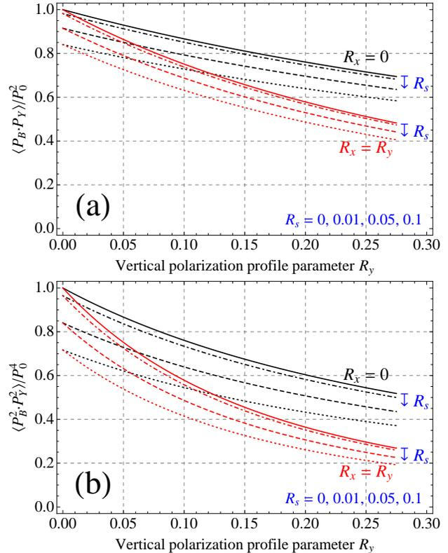
Figure 3: For double spin colliding beam experiments (a) relative reduction of the average polarization function  $\langle P_B \cdot P_Y \rangle / P_0^2$ , and (b) relative reduction of the figure of merit  $\langle P_B^2 \cdot P_Y^2 \rangle / P_0^4$ , as a function of the vertical profile parameter  $R_y$ . Assuming the same polarization profiles in both beams the cases  $R_x = 0$  and  $R_x = R_y$  are shown for  $R_s = 0, 0.01, 0.05, 0.1$  each.
