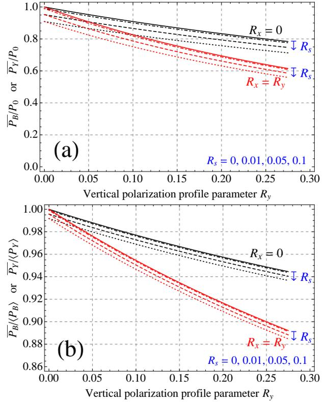
Figure 1: (a) Relative reduction of the average polarization,  $\overline{P}_B/P_0$  or  $\overline{P}_Y/P_0$ , as a function of the vertical profile parameter  $R_y$ . (b) Ratio of the polarization measured by an H-jet to the average polarization in single spin colliding beam experiments,  $\overline{P}_B/\langle P_B \rangle$  or  $\overline{P}_Y/\langle P_Y \rangle$ . The cases  $R_x = 0$  and  $R_x = R_y$  are shown for  $R_s = 0, 0.01, 0.05, 0.1$  each.
