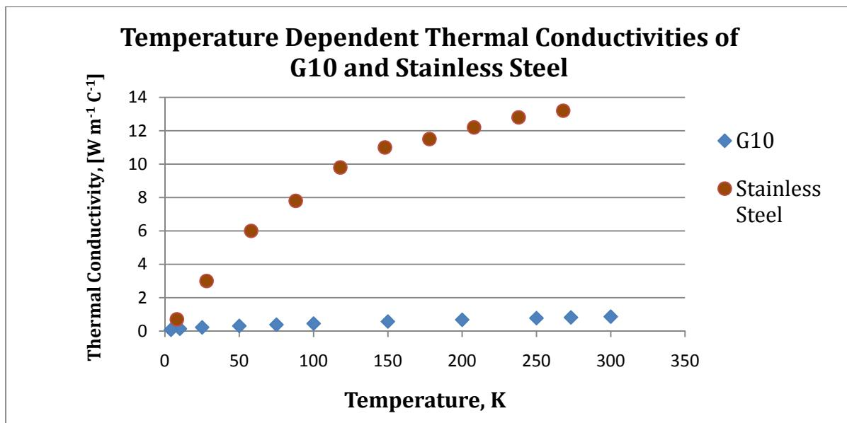
Figure 3: Temperature Dependent Thermal Conductivities<sup>4</sup>
