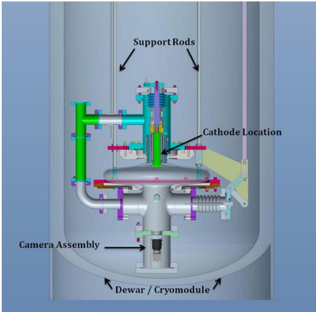
Figure 1: SRF Cavity
