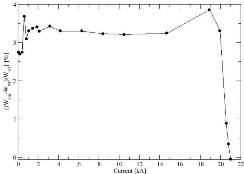
Figure 14. The percent difference between of the total energy stored in the C\_type and window-frame kickers. This percent difference in the energies stored is the same as the percent difference between the Inductances of the kickers.
