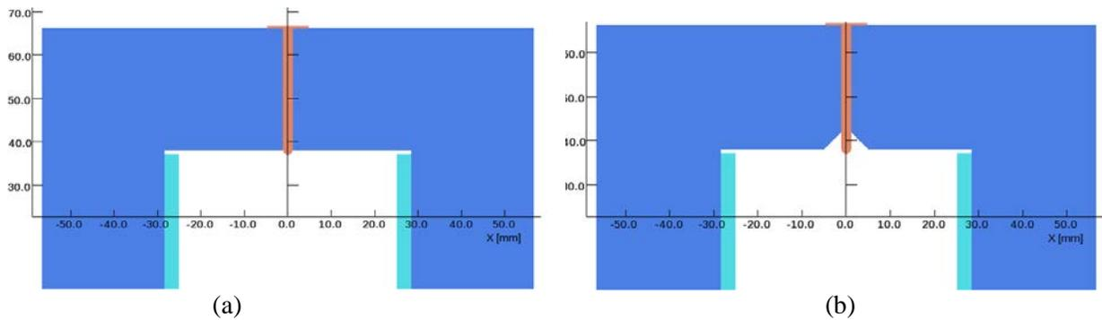
Figure 4a and 4b. The upper part of the cross section of the two possible models of the window-frame kicker to be used as RHIC-abort kickers. The comparison of the models shown in Figures 4a and 4b depicts the difference between the two possible models, one of which will be used as RHIC-abort kicker. The horizontal and vertical scales are in mm.
