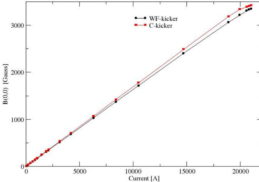
Figure 11. The black line is the plots of the magnetic field at  $(x=0,y=0)$  of the window-frame kicker shown in Figure 4b, and the red trace if the magnetic field at  $(x=0,y=0)$  of the C-type kicker, as a function of the excitation current. Both kickers are excited to the current of 21.0 [kA] in 100 nsec, with the current varying linearly with time.
