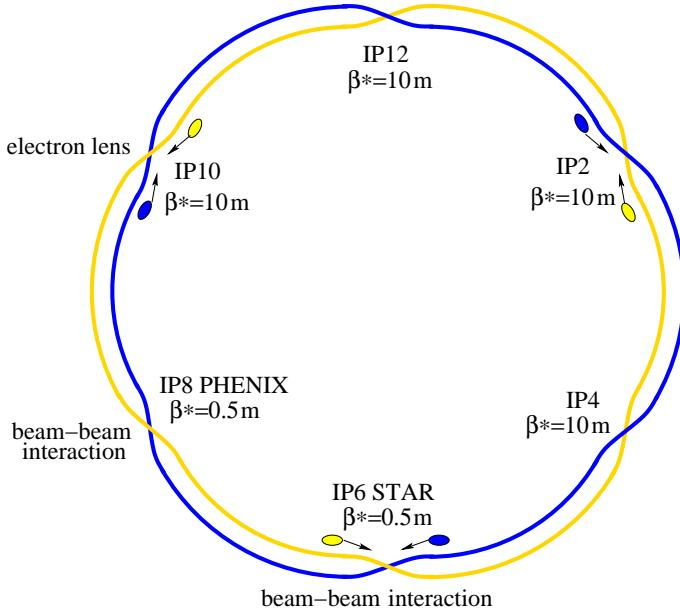
Figure 1: Layout of RHIC head-on beam-beam compensation.
