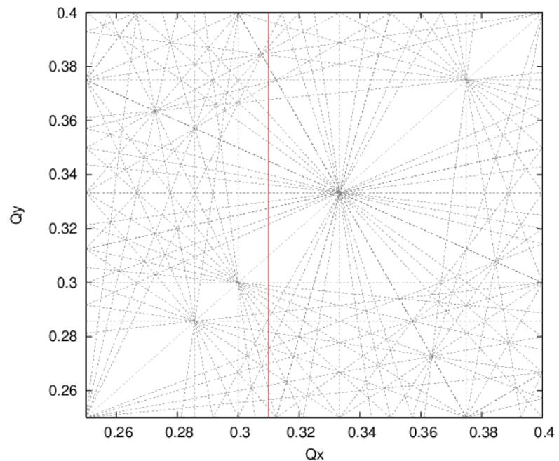
**Fig 3 Tune Diagram for 100GeV Au-Au Lattice**
