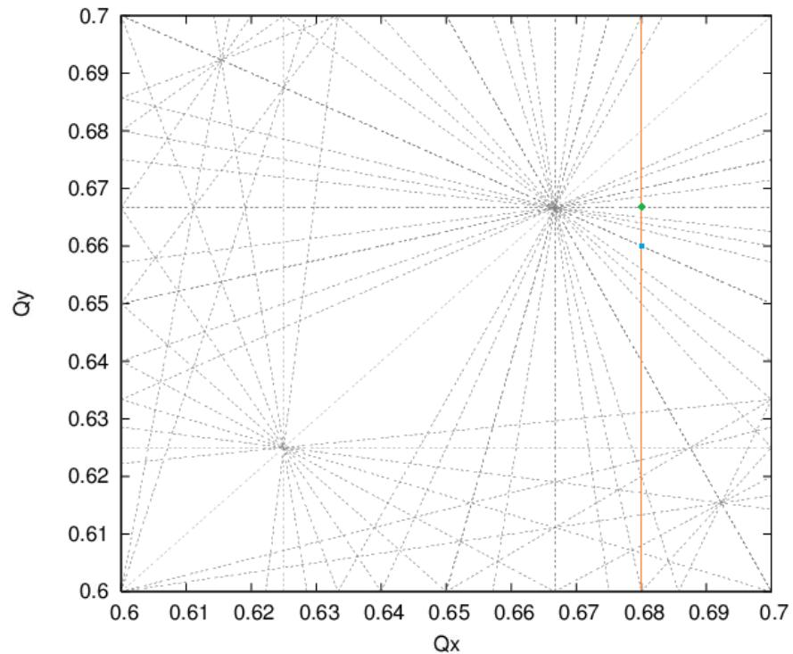
**Fig 5 Tune Diagram for 250GeV PP Lattice**
