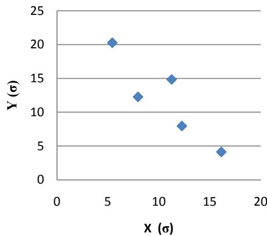
**Fig 1 Dynamic Aperture for (28.68, 29.63) 250GeV PP lattice**
