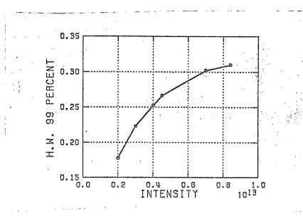
Finally, the horizontal beam size at CW100 was studied at  $2.5 \times 10^{12}$  protons per pulse for various kinds of injection tuning, with the results given below, expressed as half-width at 99% in inches.
