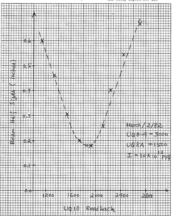
Fig. 3 Vertical beam half sizes at U618 (March 2, 1982)
