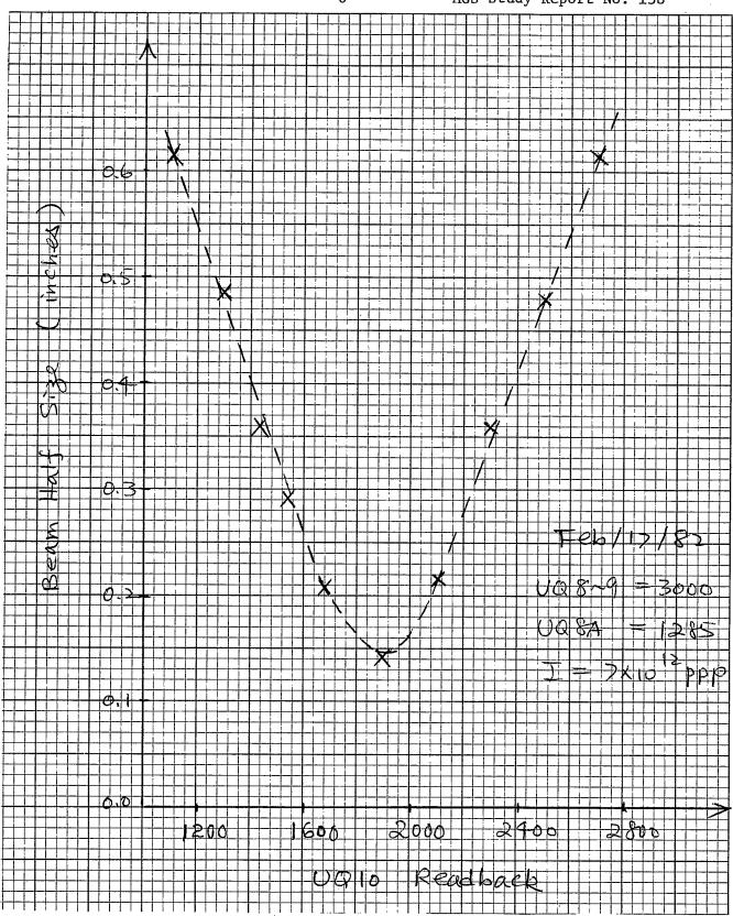
Fig. 2 Vertical beam half sizes at U618 (Feb. 17, 1982)
