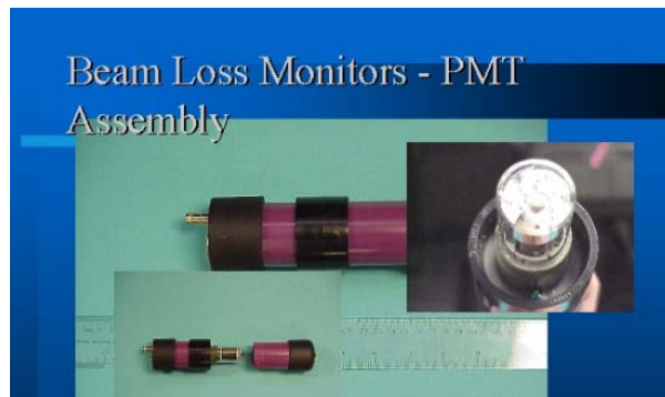
Fig. 14 PMT based BLM detector courtesy JLAB
