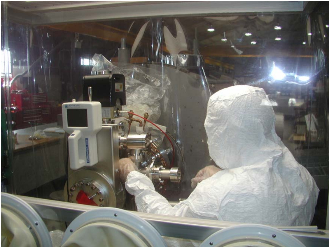
Figure 15. ERL Beamline Assembly Inside Portable Clean room
