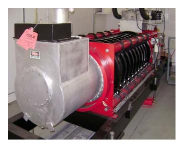
While the maximum drive specified for 1MW is 100W (40dB gain), this tube only requires 15.2W to get full power.
