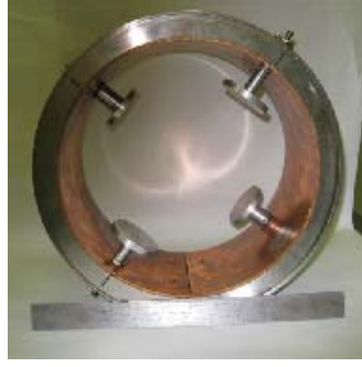
FIG. 17: Damper ring with four “mushroom” capacitive probes
