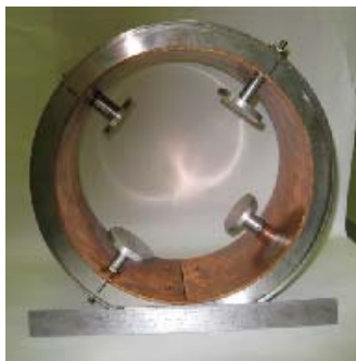
FIG. 17: Damper ring with four “mushroom” capacitive probes
