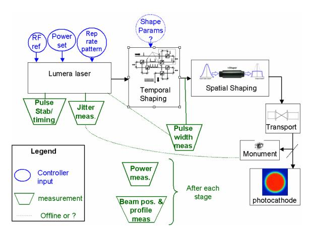
The laser is provided by a commercial vendor (Lumera). Laser timing and rep. rate signals will be derived from the master RF system clock. The RF clock system will provide pulse patterns to support diagnostic modes and intensity "ramp up" - to gradually increase the pulse train width over time to avoid excessive "droop" in the energy recovery cavity.
