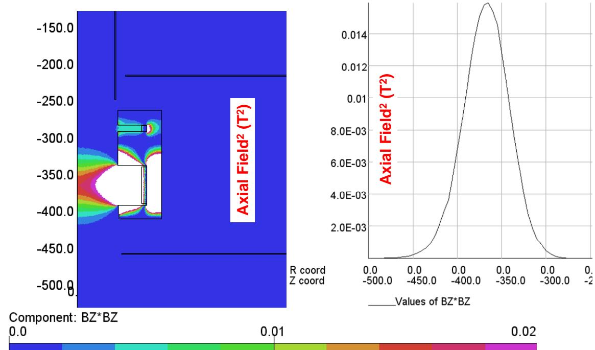
Fig. 1.4. Computed map of the focusing ( $B_z^2$ ) is shown on the left and the axial profile of the focusing ( $B_z^2$ ) along the beam axis is shown on the right.
