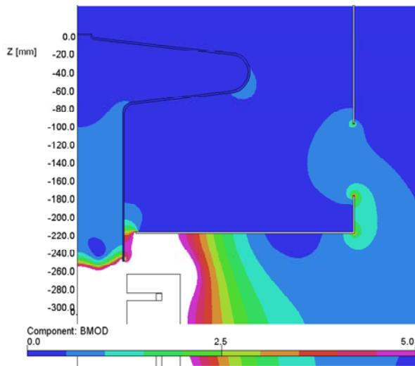
Field inside cavity with bucking coil turned off
