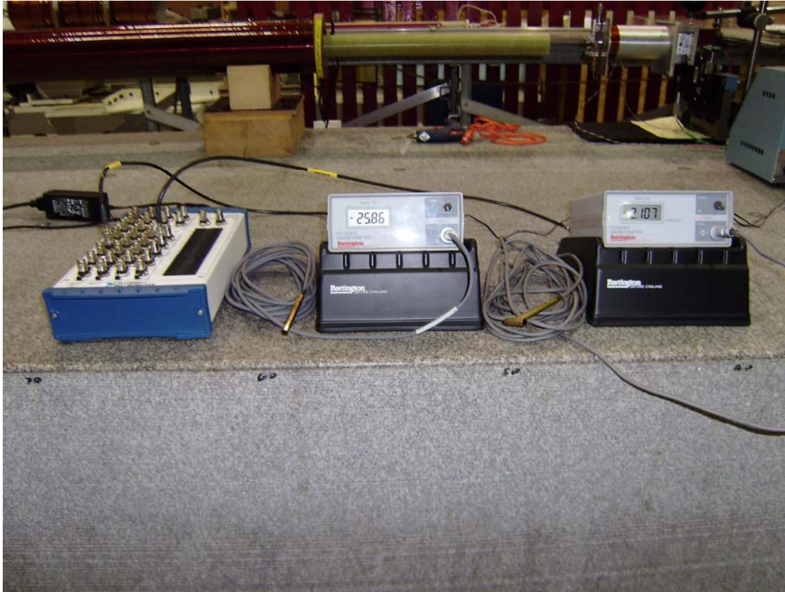
Fig. 3. 5. Fluxgate magnetometers with axial probe (left) and transverse probe (right) and the NI USB ADC /connector unit (far left).
