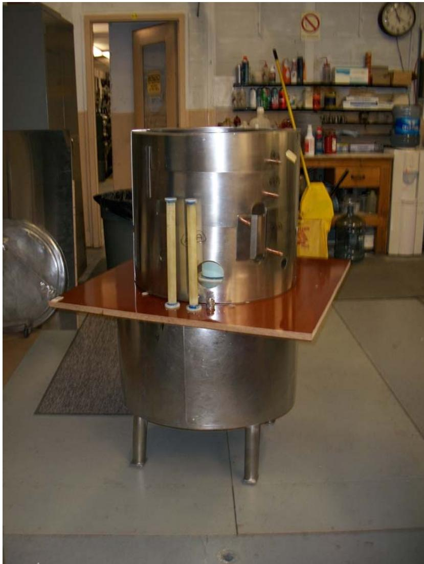
Fig. 3.4. Test cryostat with shield in place.
