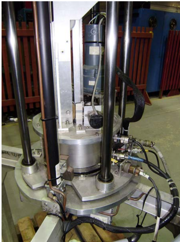
Figure 3.2. Close up vertical transporter drive mechanisms.
