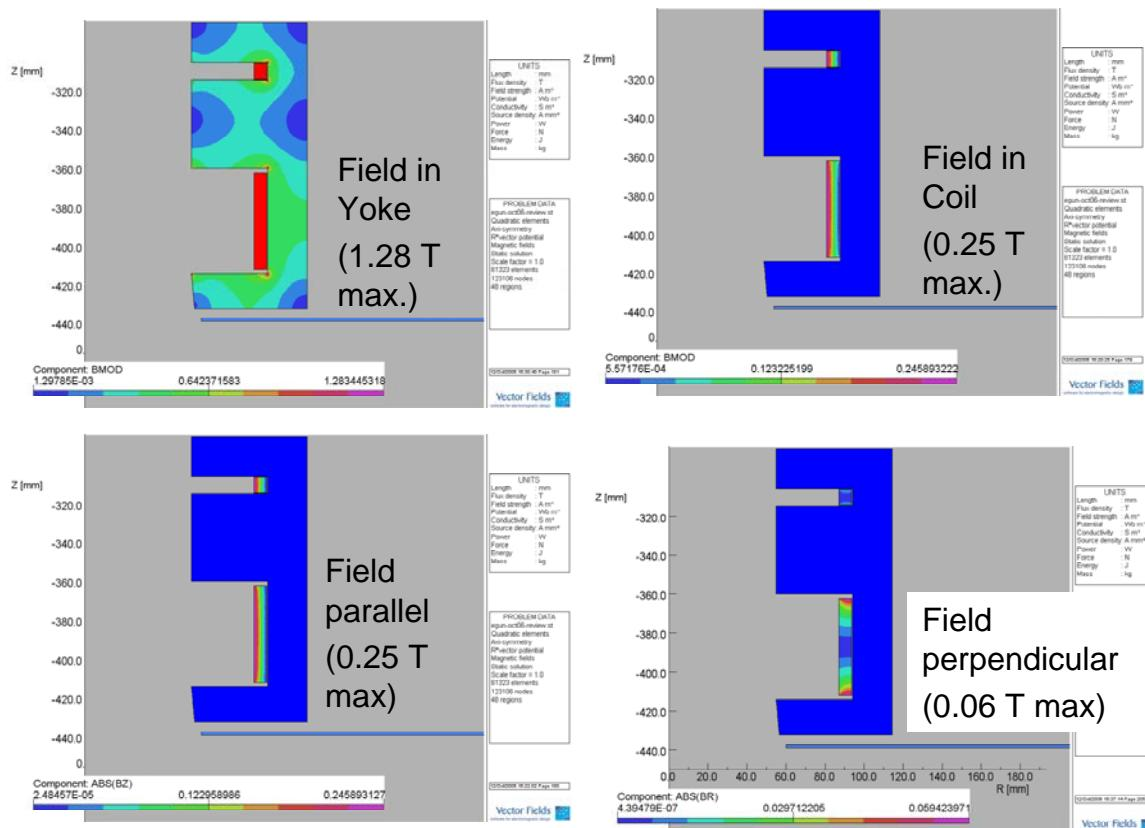
Fig. 1.13. Parallel and perpendicular components of the fields on surface of HTS tape in the presence of yoke iron. One can see that the iron has significantly reduced the perpendicular component of the field (compare to the case of no iron in Fig. 1.12), increasing the critical current of the solenoid.
