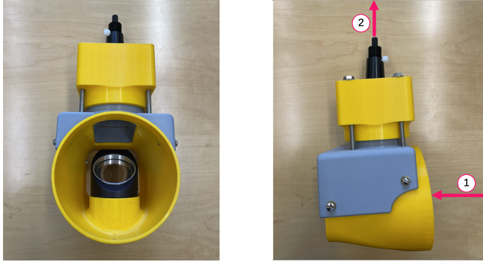
(a) View along light path onto the Polka dot mirror. (b) Sideview, Polka dot mirror deflects light coming from the right (1) upon exiting the viewport by 90^\circ to the collection lens, where the fiber glass cables are connected (2), which are transporting light to the spectrometers in the bldg. 1012.
