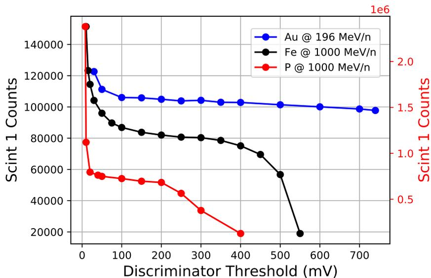
Figure 2: Raw scintillator counts as a function of discriminator threshold magnitude for beams considered in this study.
