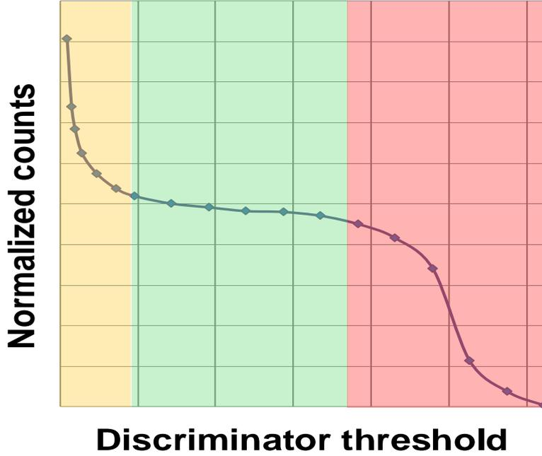
Figure 1: Generalized overview of a discriminator threshold curve and the referenced sections of the curve. The orange section encompasses the region of high scintillator noise. The green center section encompasses the plateau or flat region where scintillator counts are independent of set point. The final red section represents the region where the voltage set points are above the threshold for ion detection.
