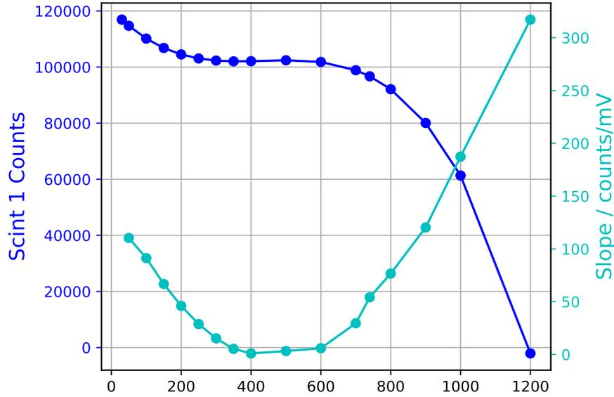
Figure 5: Derivative of the discriminator threshold curve for the Au @ 196 MeV/n beam.
