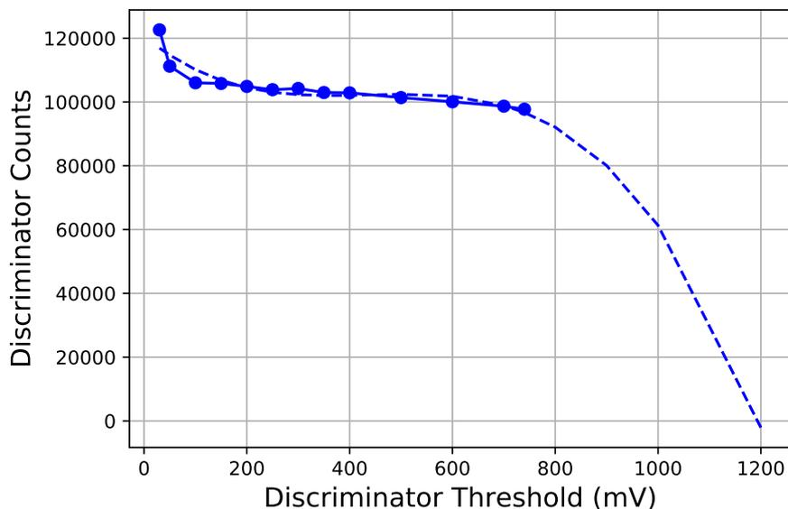
Figure 3: Raw scintillator counts and the extrapolated discriminator curve for Au @ 196 MeV/n.
