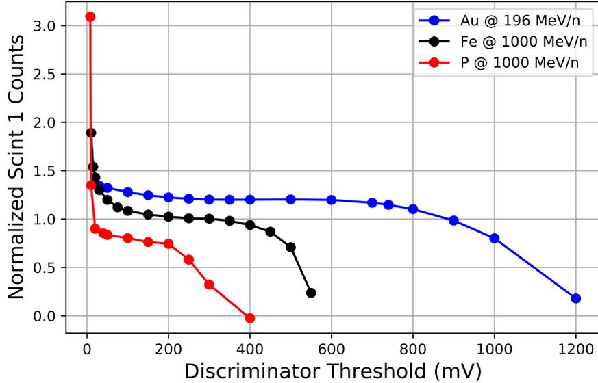
Figure 4: Discriminator counts as a function of discriminator threshold setting for each beam. The discriminator counts are normalized by the mean value of the “plateau” region of each curve. The P @ 1000 MeV/n and the Au @ 196 MeV/n curves are shifted vertically for visualization purposes.
