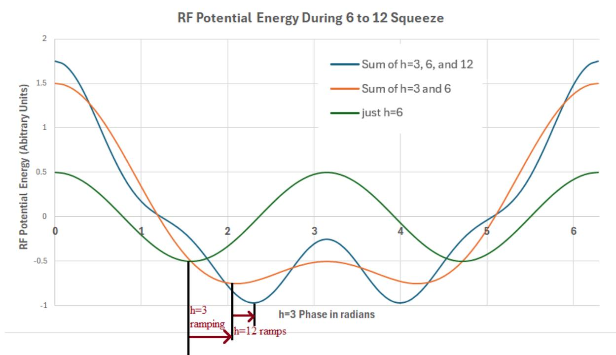
**Figure 3:**  $U(\varphi)$  at different points in the squeeze. The green trace is where only  $h=6$  voltage is present, the orange trace is where  $h=3$  has also been ramped, and the blue trace is where  $h=12$  has also been ramped (to some degree).
