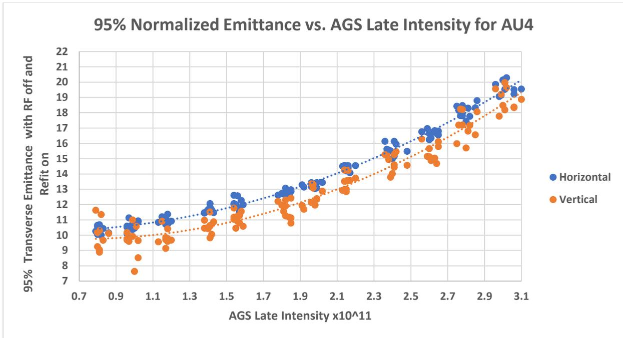
**Figure 14:** AGS IPM transverse 95% normalized emittances as a function of AGS Late for the standard BU4/AU4 setup (snakes on, tune jump quads on) in  $\pi$  mm mr. The dashed lines are quadratic fits to the data,  $\epsilon_x=1.44N^2-1.39N+10.61$  and  $\epsilon_y=1.68N^2-2.38N+10.60$ , where  $N$  is AGS Late. The intensity was varied by adjusting the Linac pulse width with a constant amount of scraping.
