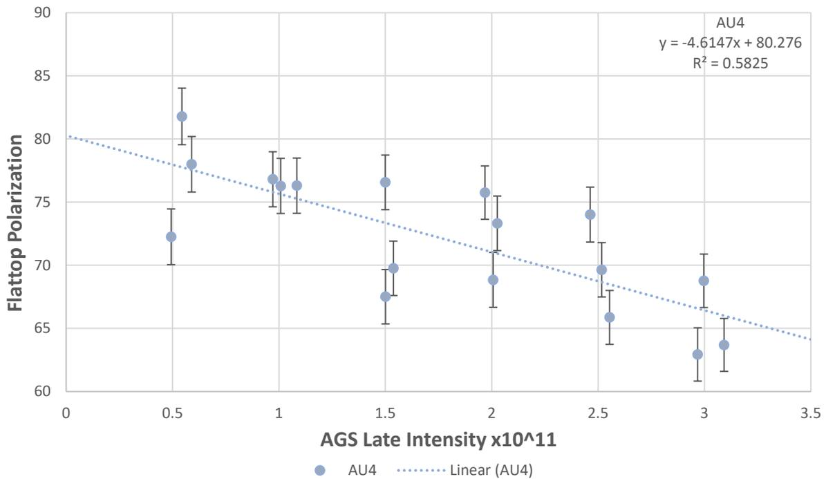
**Figure 25:** The AGS Flattop Polarization vs. AGS Late intensity scans for AU4 together with a linear fit,  $P(I) = -4.6147(I) + 80.276$ . Intensity was varied using vertical scraping and the pulse width was set to 300  $\mu$ s. Vertical target 3 was used. The error bars are +/- the ErrFit parameter in the Krisch display. The data was taken on Aug. 24<sup>th</sup> by T. Dankworth.
