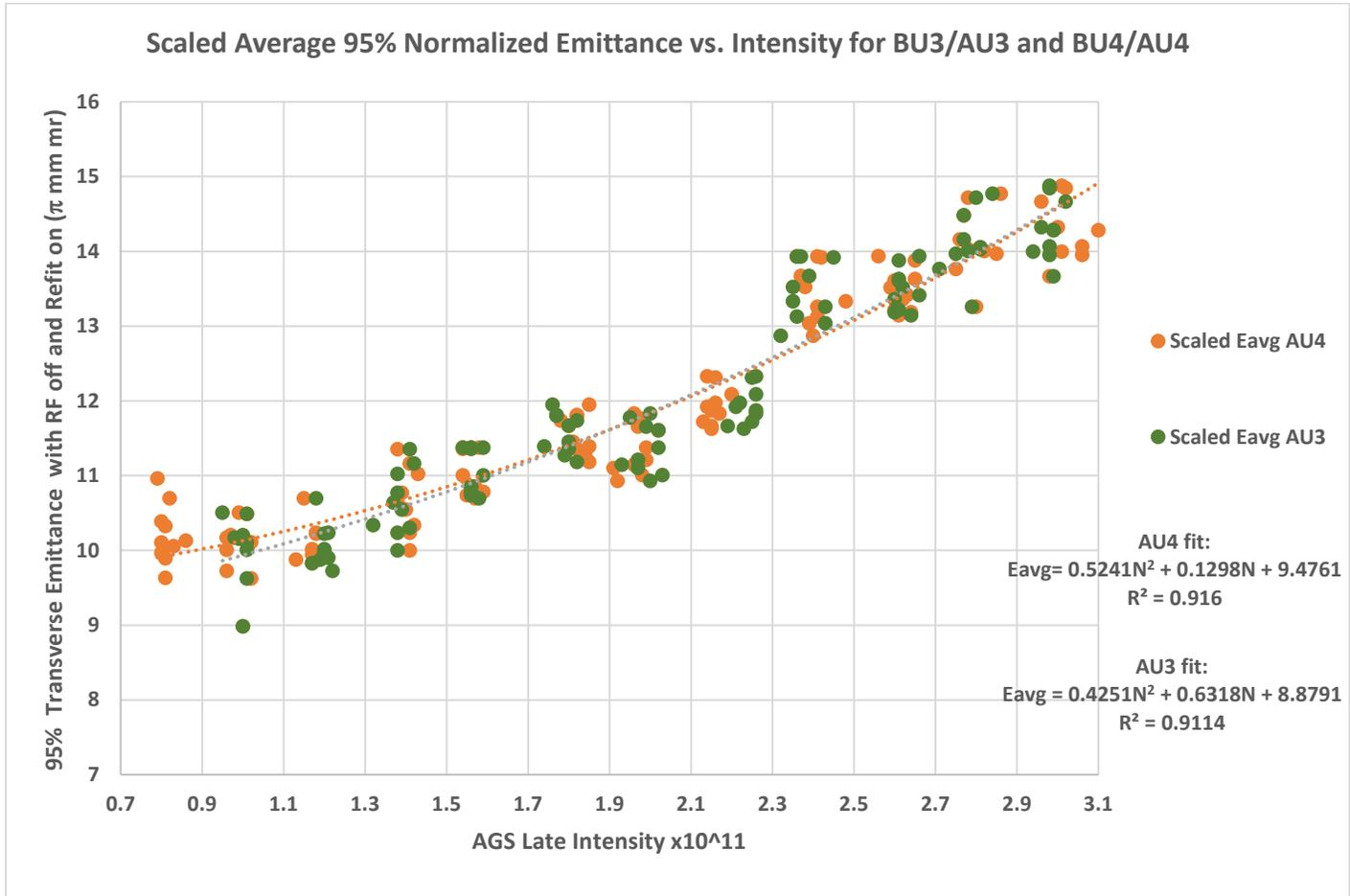
**Figure 18:** The average emittance, defined as  $E_{avg} = \sqrt{(\epsilon_x^{*2} + \epsilon_y^{*2})/2}$ , for the AU3 and AU4 flattop emittance data where  $\epsilon_x^*$  and  $\epsilon_y^*$  are  $\epsilon_x$  and  $\epsilon_y$  scaled by the BtA MW006 emittance growth.
