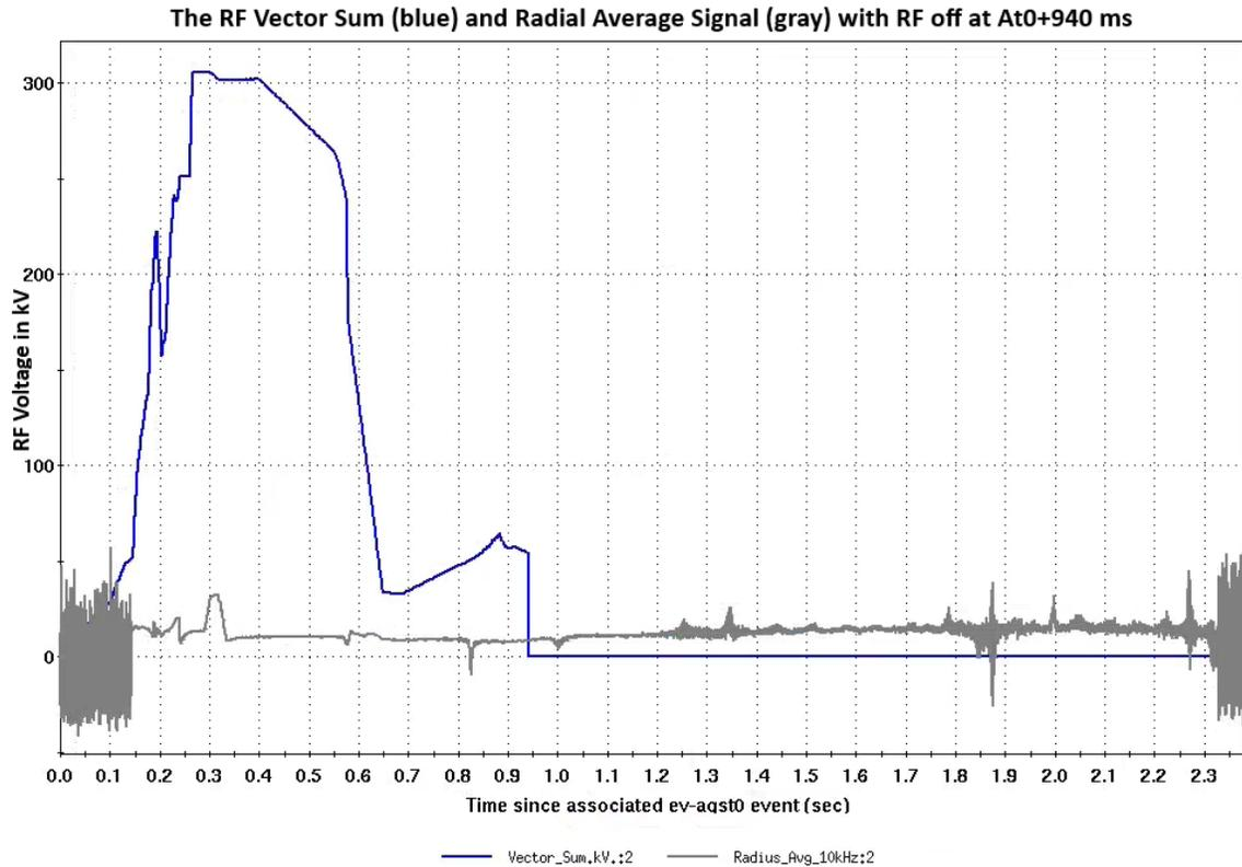
**Figure 12:** The vector sum (*Vector\_Sum.kV*, in blue) and radial average signal (*Radial\_Avg\_10kHz*, in gray) on AU3 with RF shutting off at 940 ms and an AGS Late of about  $3e11$ . Taken from *AgS/RF/LLRF/agsDspAll.logreq*. It is the cycle on Sept. 23, 2024 that starts at 17:44:09.<sup>35</sup>
