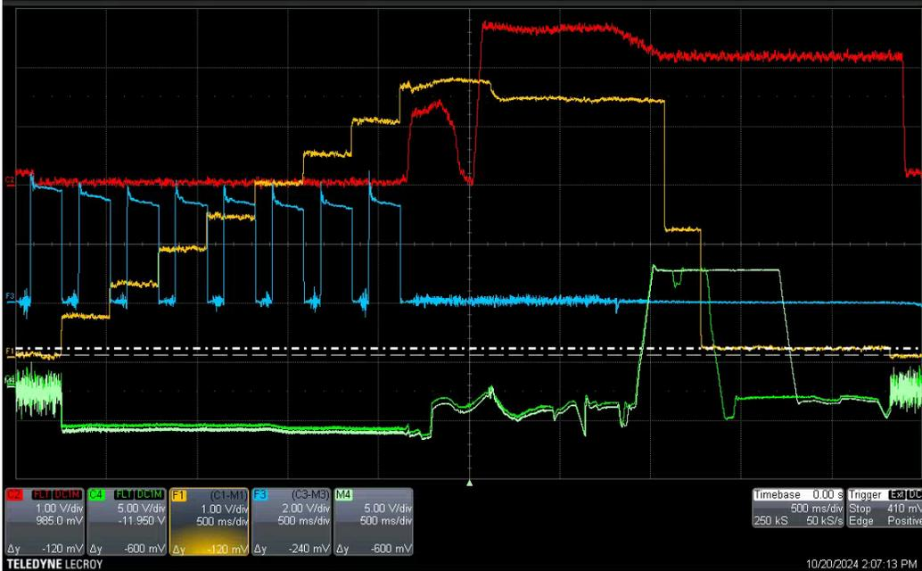
**Figure 31:** The AGS cycle with the 12-6-3 merge. F1 is the normalized current transformer (with baseline subtracted, orange), the red trace is the RF detected vector sum, the green traces are the G09 horizontal BPM with the G09 bump on long enough for 2 extractions (C4) and for 4 extractions (M4). The trigger is At0+2300 ms and the sweep speed is 500ms/div. AGS Late is about 5e9.
