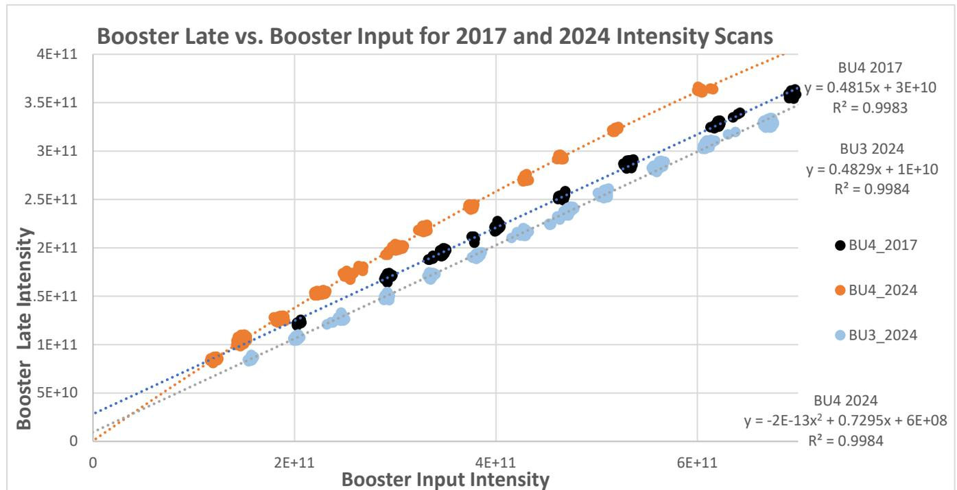
**Figure 21:** Booster Late vs, Booster Input for the Flattop emittance scans this run (BU3 in blue and BU4 in orange) and in 2017 (black) together with fits, linear for BU3 and 2017 BU4 and quadratic for BU4 this run.
