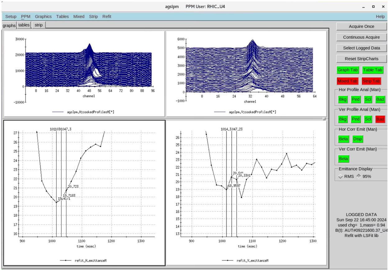
**Figure 13:** A set of AGS IPM measurements on AU4 with  $3.0e11$  AGS Late and RF shutting off at 940 ms. The vertical cursor lines indicate which data points are used for the measurements (1014, 1030.5, and 1047 ms). This logged data is from Sept.22 2024, 16:45:00 and it uses Refit.
