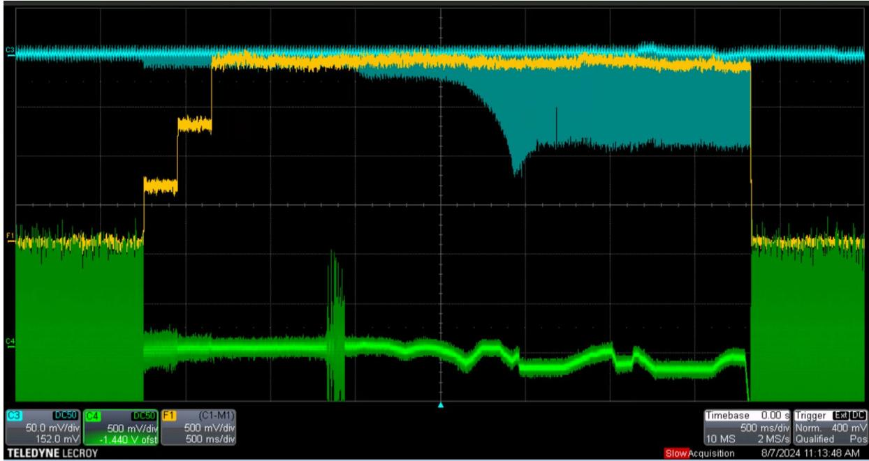
**Figure 29:**  ${}^3\text{He}^{2+}$  in the AGS with 3 transfers. The A15 normalized current transformer (orange), the wall current monitor (blue), and the J12 horizontal BPM (green). The trigger is At0+2000 ms. The AGS Late intensity here is about  $1.3e10$ .<sup>61</sup>
