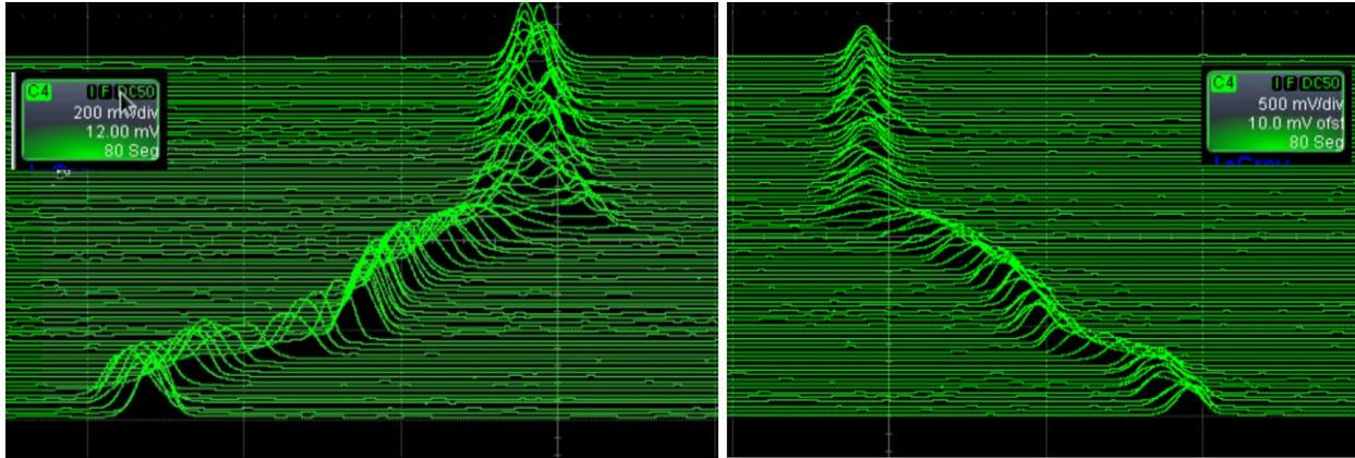
**Figure 4:** WCM mountain range display of the squeeze and merge with only 1 Booster transfer. Only the first transfer is on the left and has a gain of 200mV.div. On the right is just the second transfer, which has a gain of 500 mV/div. The sweep speed is 100ns/box in both cases. Looking at 80 traces from 1650 to 3050 ms.
