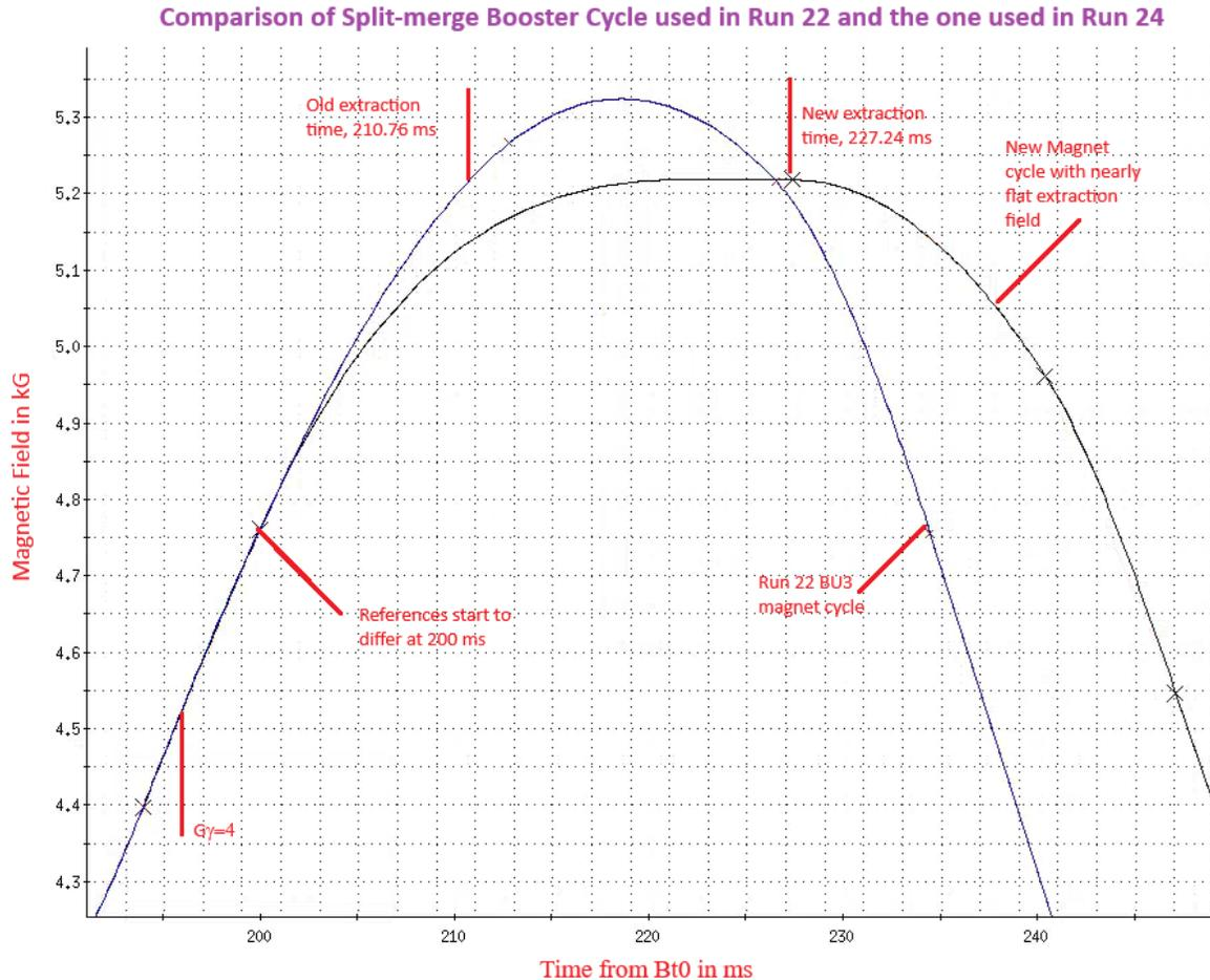
**Figure 10:** Comparison of the Booster magnet references used in Run 22 and 24 showing that, in Run 24, extraction occurs when the field is nearly flat which allows the RF voltage to be lowered more than in Run 22 to reduce their peak current.
