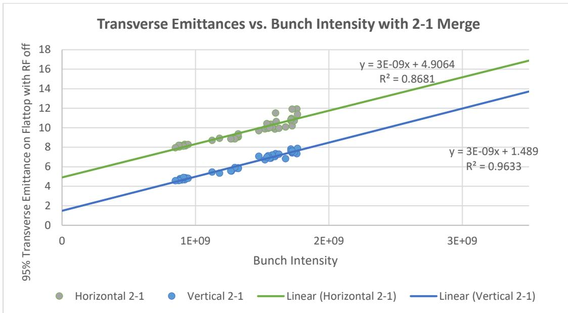
**Figure 32:** Flattop 95% IPM transverse emittances vs. flattop bunch intensity using the 12-6 (2-1 type) merge where the pulse width is varied to change the bunch intensity. Emittances are in units of  $\pi$  mm mr.
