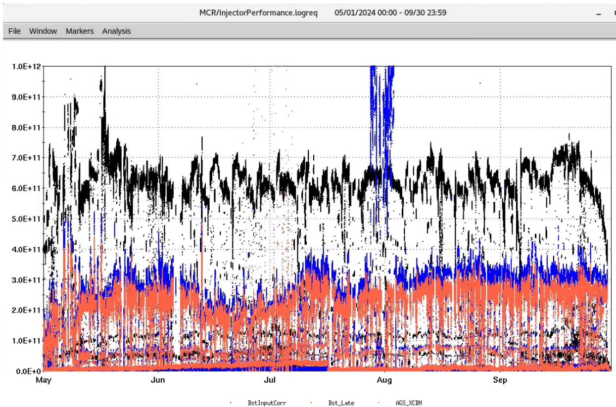
**Figure 20:** The “adjusted” Booster Input (black), Booster Late (blue), and AGS Late (red) intensity scalers during the PP run (May 1 to Sept. 30). The “adjusted” Booster Input is the actual Booster Input multiplied by 0.94.
