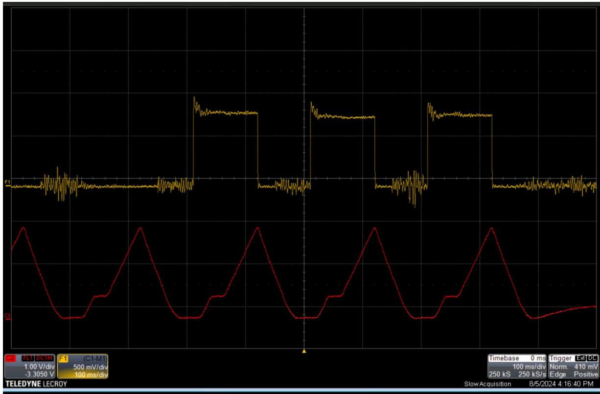
**Figure 28:** The 3 Booster  $^3\text{He}^{2+}$  cycles with beam as viewed on the normalized circulating transformer (orange) and the Booster main magnet current showing the 5 magnet cycles (the first 2 are the dummy cycles). The trigger is Bt0 on cycle 4. The Booster late is about  $1.3 \times 10^{10}$  and Booster input (xf108 sum) is about  $2.4 \times 10^{10}$ .<sup>59</sup>
