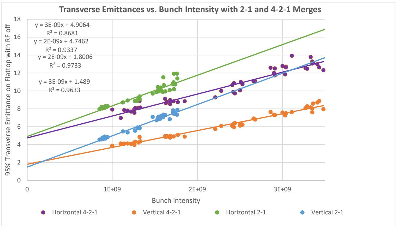
**Figure 34:** 95% IPM transverse emittances vs. flattop bunch intensity using the 12-6-3 and 12-6 merges where the pulse width is varied to change the bunch intensity. Emittances are in units of  $\pi$  mm mr.
