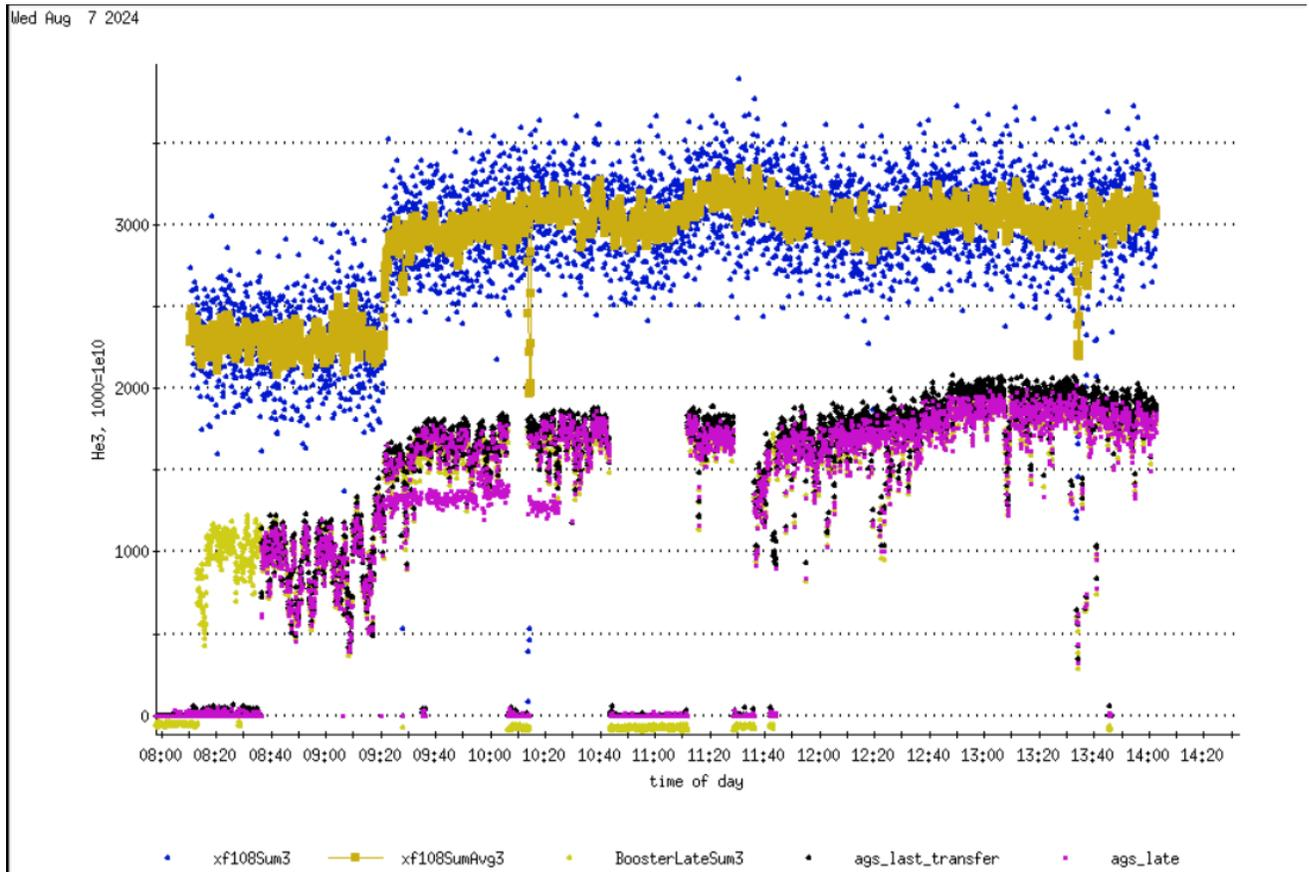
**Figure 27:** Intensity scalers for He3 on the day of the APEX experiment. Xf108Sum3 (blue) is the sum of the 3 EBIS pulses at xf108, xf108Sum3Avg (dark yellow) is a 10 supercycle running average of xf108Sum3, BoosterLateSum3 is the Booster Late intensity (lighter yellow), ags\_last\_transfer is the AGS intensity on the injection porch after the last transfer (black), and ags\_late (purple) is the intensity just before extraction time (3300 ms).
