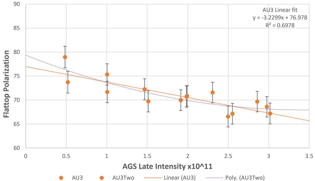
**Figure 26:** The AGS Flattop Polarization vs. AGS Late intensity scans for AU3 together with a linear fit,  $P(I) = -3.2299(I) + 76.978$  (orange). A quadratic fit is also shown in faint purple. Intensity was varied using vertical scraping and the pulse width was set to 300  $\mu$ s. Vertical target 3 was used. The error bars are +/- the ErrFit parameter in the Krisch display. The data was taken on Aug. 24<sup>th</sup> by T. Dankworth.
