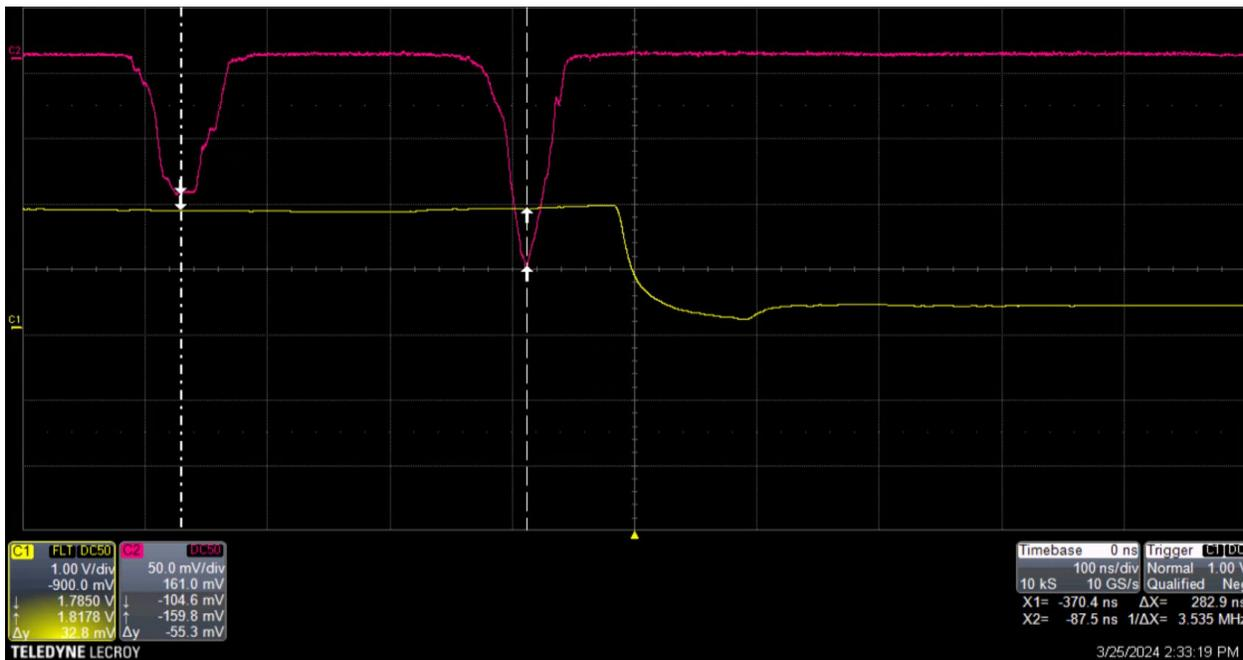
**Figure 5:** The first (left) and second (right) transfers on the WCM (red trace) at At0+1850 ms. The bunch from the first transfer is much larger than the one from the second because it was not well matched at injection and beam control is not on before the 2<sup>nd</sup> transfer. 100 ns/div. The yellow trace is the Rev tick. Also, the bunches are 283 ns apart.
