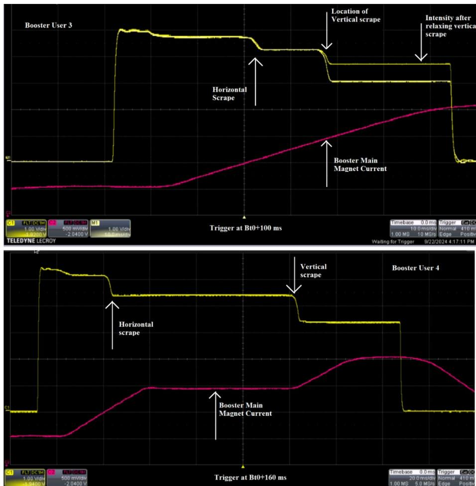
**Figure 19:** The horizontal and vertical scrapes used for the scans on BU3 (bottom) and BU4 (top). The yellow traces are the Booster normalized current transformer. The AGS Late intensity in both cases is about 3.0e11 and the Linac pulse width is 300  $\mu$ s. The sweep speed for the top plot is 20 ms/div and it is 10 ms/div for the bottom plot. The red traces are the Booster magnet current. The yellow traces are 1V/div.
