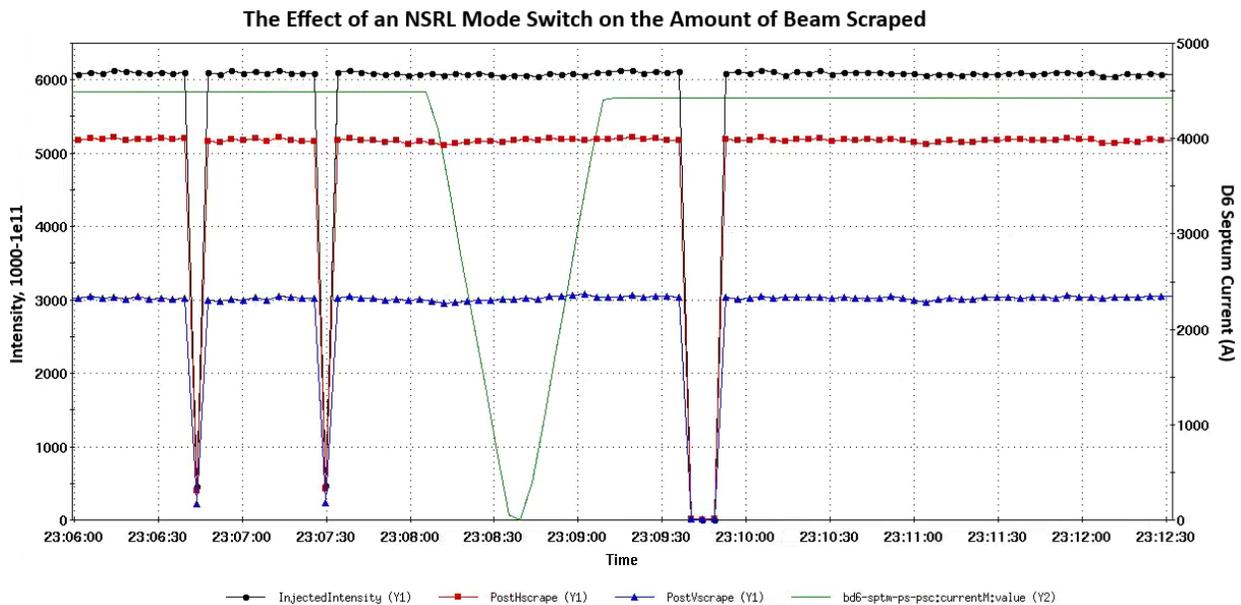
**Figure 23:** The intensity just after injection (black), just after the horizontal scrape (red), and just after the vertical scrape (blue) together with the D6 current (green, y-axis on right) during an NSRL mode switch on Sept. 16<sup>th</sup>.
