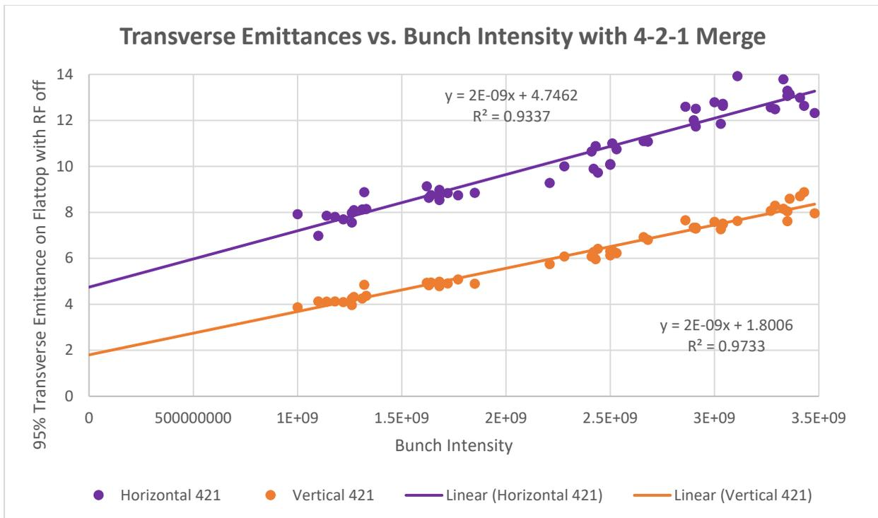
**Figure 33:** 95% IPM transverse emittances vs. flattop bunch intensity using the 12-6-3 (4-2-1 type) merge where the pulse width is varied to change the bunch intensity. Emittances are in units of  $\pi$  mm mr.
