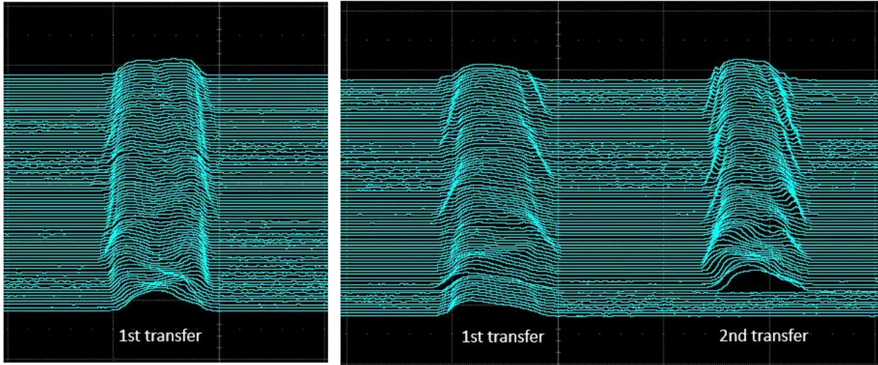
**Figure 6:** WCM Mountain range displays for the 10 ms after the first transfer (left) and for 10 ms after the 2<sup>nd</sup> transfer showing both bunches (right).
