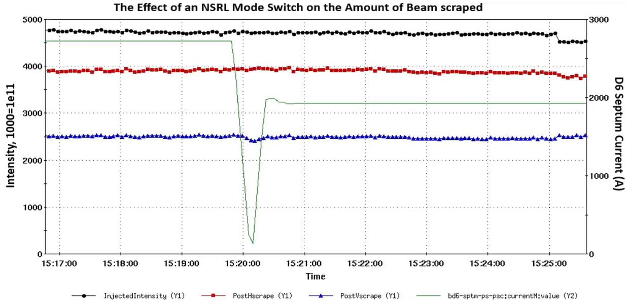
**Figure 24:** The intensity just after injection (black), just after the horizontal scrape (red), and just after the vertical scrape (blue) together with the D6 current (green, y-axis on right) during an NSRL mode switch on Sept. 5<sup>th</sup>.
