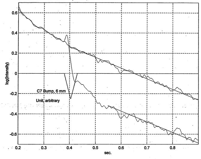
28-Apr-1998, Gold Beam Life Time vs. Beam Loss
