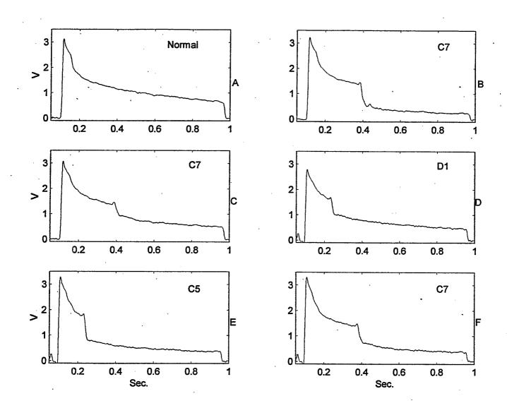
Fig.1. Beam scraped at C7, C5, and D1. The case A is a normal cycle.
