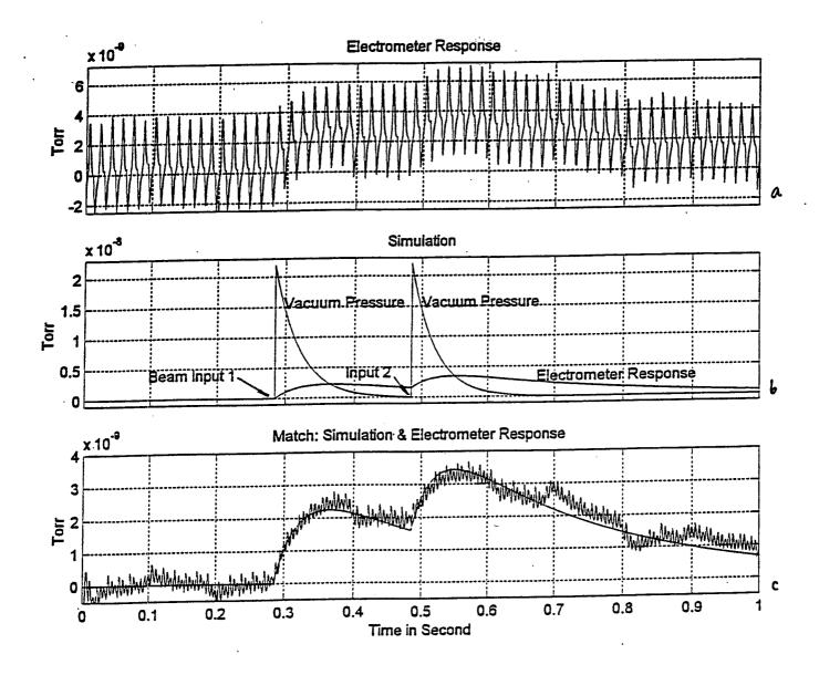
Fig.2: Experiment II. Simulated vacuum pressure decay time is 35 ms.
