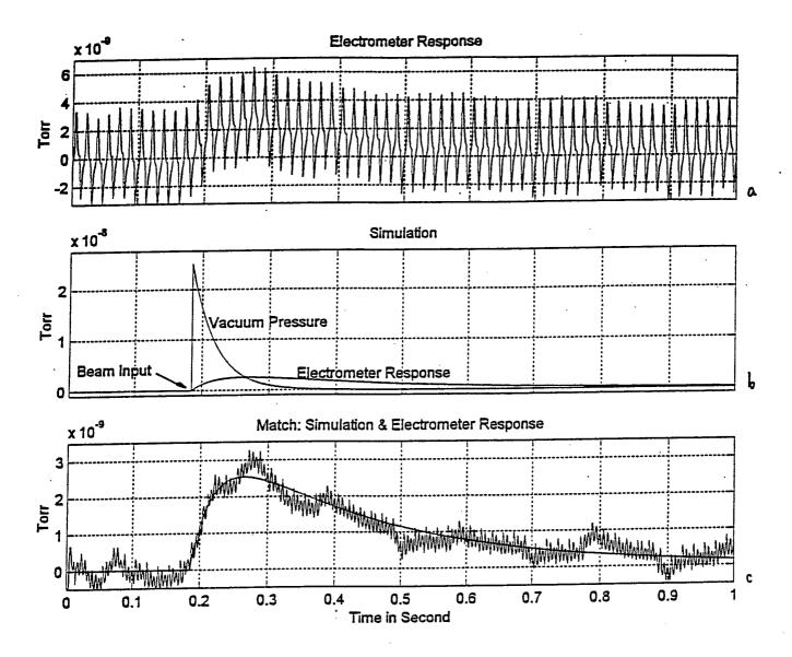
Fig.1: Experiment I. Simulated vacuum pressure decay time is 35 ms.
