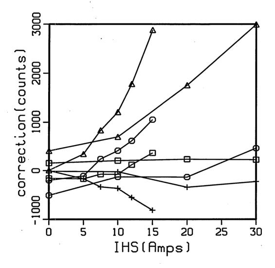
Figure 1: SN26 corrector settings .vs. current in the horizontal chromaticity sextupoles. square(VB,-VE,VH,-VK); circle(VC,-VF,VI,-VL); triangle(HB,-HE,HH,-HK); cross(HC,-HF,HI,-HL)
