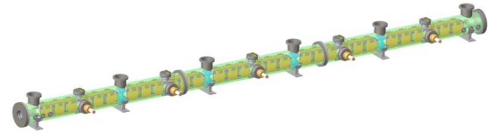
Figure 2: Chamber of Five Kicker Magnets' Assembly
