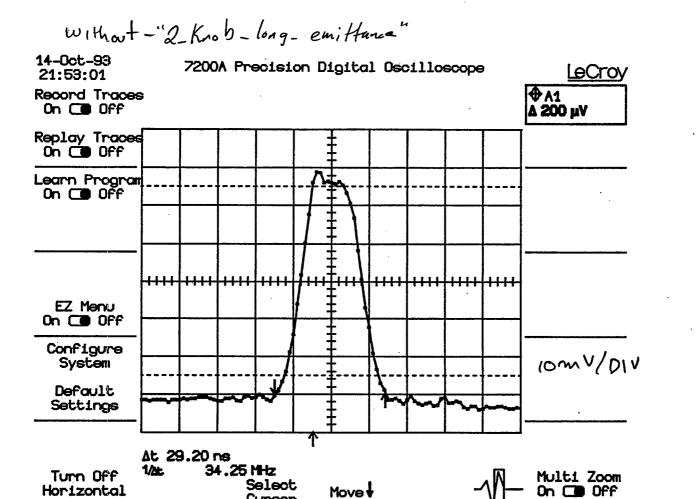
Figure 7: The bunch shape in the normal rf program.
