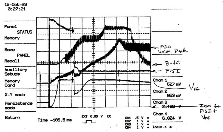
Figure 3: Voltage program 1. F15 current transformer signal (beam intensity). The rate of change of magnetic field  $\dot{B}$ . F20 wall current monitor signal (bunch shape).
