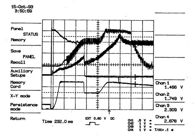
Figure 6: Voltage program 2. F15 current transformer signal (beam intensity). The rate of change of magnetic field  $\dot{B}$ . F20 wall current monitor signal (bunch shape).
