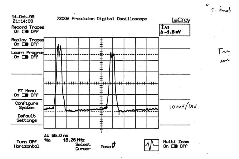
Figure 4: The bunch shape in the normal rf program.
