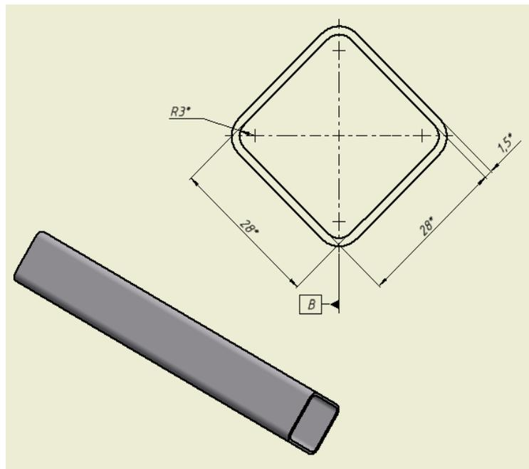
Figure 1: Cross-section of the wiggler vacuum chamber.
