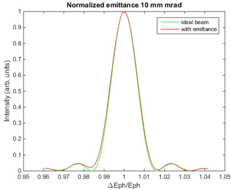
Figure 3: Change of the planar undulator radiation spectrum due to the angular spread caused by emittance (no dispersion). The beam energy is 275 GeV ( $\gamma=293.1$ ), and the angular spread corresponds to the  $\beta$ -function of 1 meter. The angular spread causes a redshift of the spectrum (here  $\Delta E_{ph}/E_{ph}=1.29 \times 10^{-3}$ ) and the red curve is shifted for clarity.
