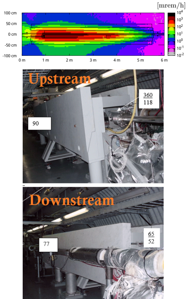
FIG. 3. Top panel: Plan view of H^*(10) [mrem/h] for the blue dump at 1 day post EOB calculated with FLUKA. Beam travelled from left to right and the dose rates are averaged over 10 cm, centered at beam level. Lower panels: excerpted from the radiological survey report at 1 day post EOB, all survey values are in mR/h and general area doses except for the values underlined, which are contact readings.
