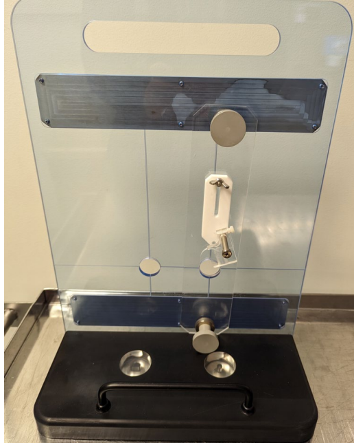
Figure 9: Target fixture for SOBP. Target can be mounted, via bite bar, and attached to vertical surface by two magnets.
