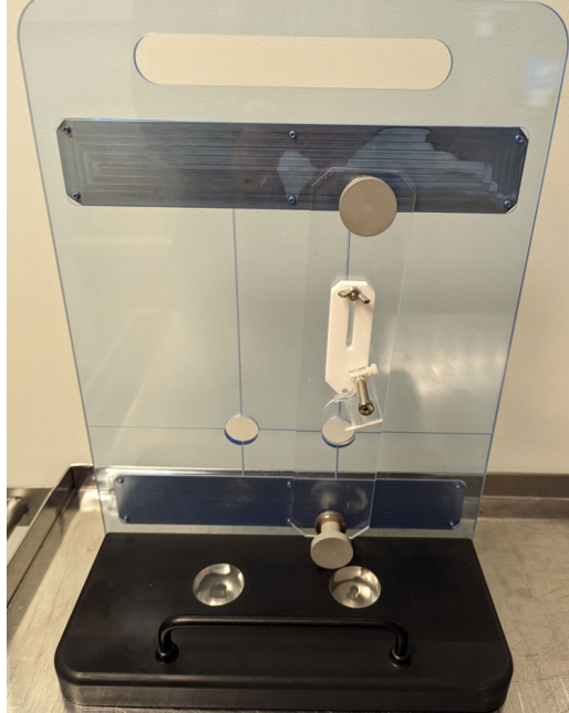
Figure 9: Target fixture for SOBP. Target can be mounted, via bite bar, and attached to vertical surface by two magnets.
