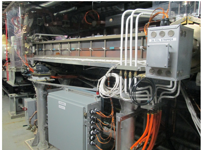
FIG. 3: Physical D6 septum magnet with foil stripper at the beginning of the NSRL transport line.
