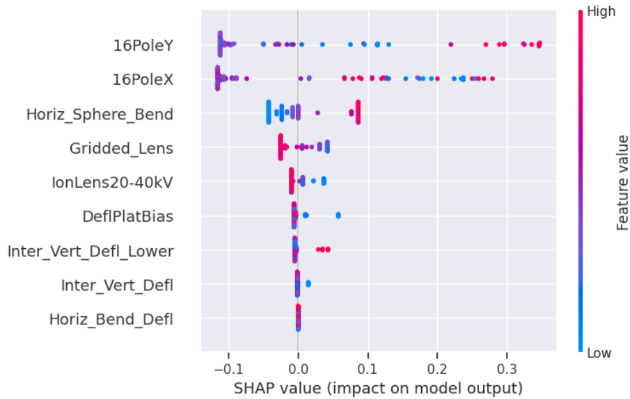
Fig. 11: The importance of individual feature/parameter for the injection beam line.
