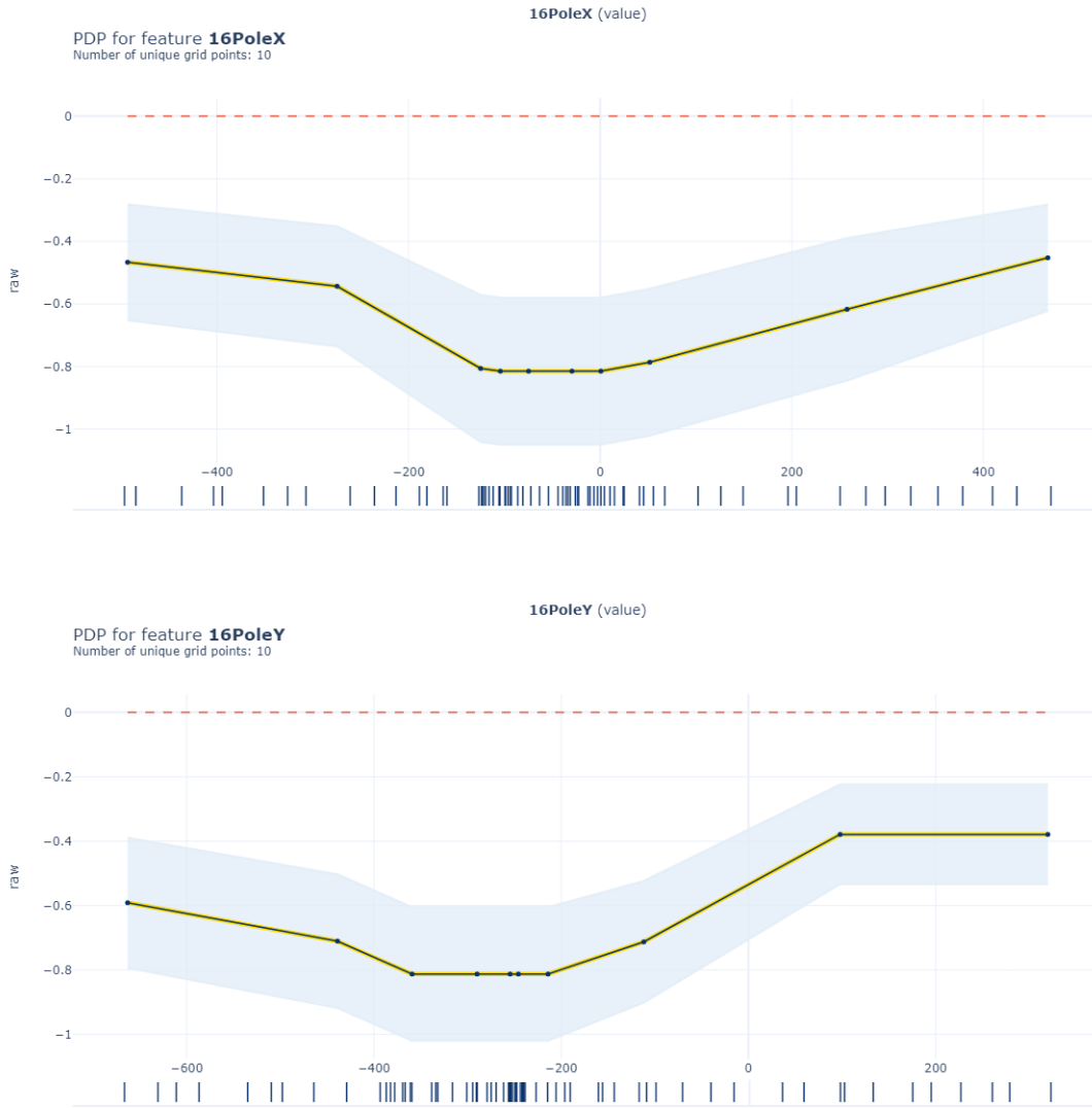
Fig. 15: The partial dependence plot for 16PoleX (top) and 16PoleY (bottom) in the injection line.
