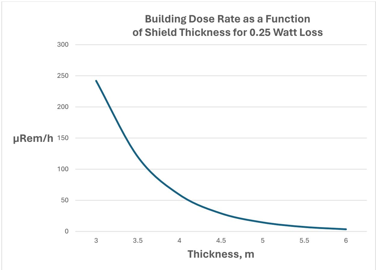
The 0.25 Watts of HSR beam losses are the controlling factor for the soil berm shielding. The 4.1 meters required is larger than the 2.3 meters required for 0.5 Watts of ESR beam losses. Both beam powers are considered order-of-magnitude estimates of routine beam losses in the 1010 sector of the ring, which is unavoidable and chronic.
