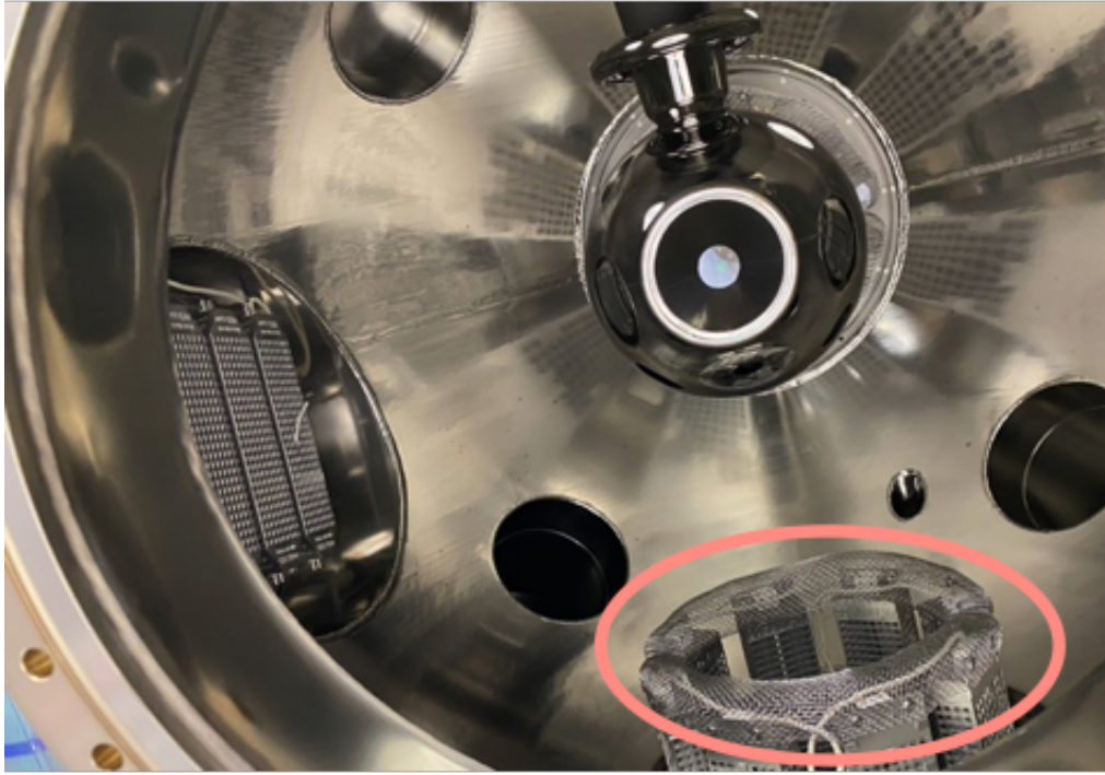
Figure 4. The circled area shows the mesh covering the top of the NEG pump.
