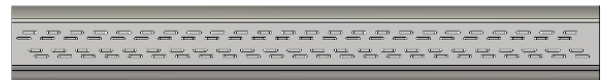
FIG. 1. Model used to compute resistive-wall heating (top) and top view of screen with array of pumping slots (bottom).
